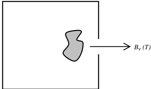
**Fig.4.6: Blackbody radiation coming out of a box with an optically thick obstacle placed behind the hole inside the box**
