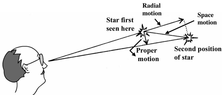
Fig.1.7: Radial and proper motion of a star
