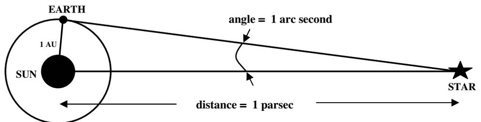
Fig.1.1: Schematic diagram showing the definition of 1 parsec. Note that  $1^\circ \equiv 60'$  and  $1' = 60''$ . Thus,  $1'' = 1/3600$  degree
