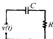
Fig.13.6: An RC circuit
