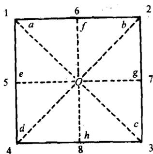
Fig.5.6: The axes and planes of symmetry of a square
