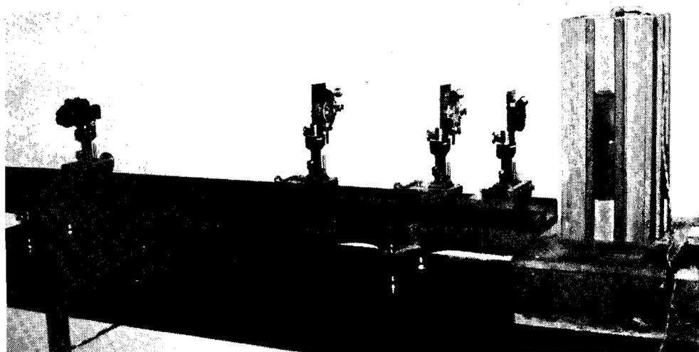
Fig. 2.4: The experimental setup for observing interference pattern due to Fresnel's biprism.
