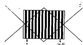
Fig. 2.5: Enlarged view of the fringe pattern. Note how the intersection of the cross-wires is placed on any (here  $n^{\text{th}}$  fringe) bright fringe.
