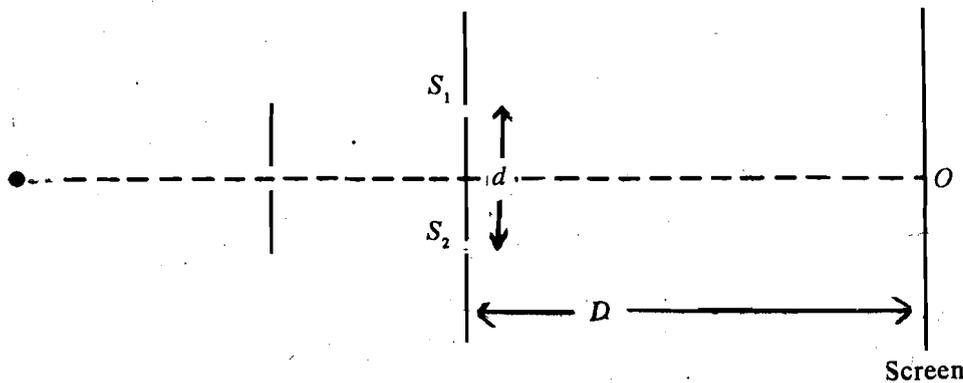
Fig.2.1: Cross-sectional view of the double slit arrangement to observe interference of light waves
