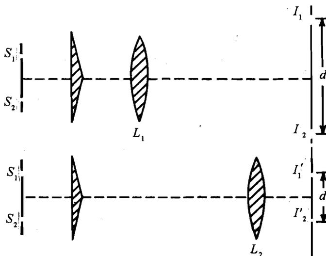
Fig.2.3: Two positions of the lens between the biprism and the eye-piece giving enlarged images  $I_1, I_2$  and diminished images  $I'_1, I'_2$  of  $S_1$  and  $S_2$
