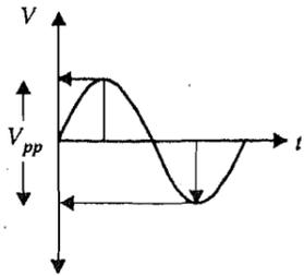
Fig. 13.7 : Voltage measurement.
