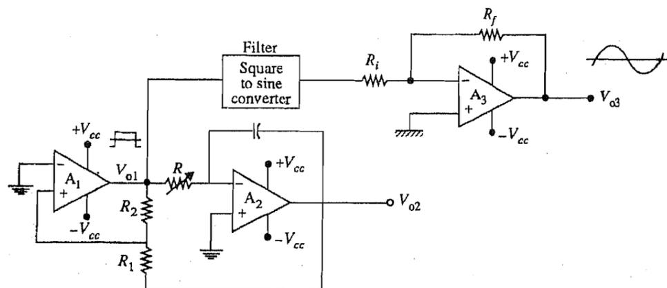
Fig.13.10 : Circuit of a basic function generator.
