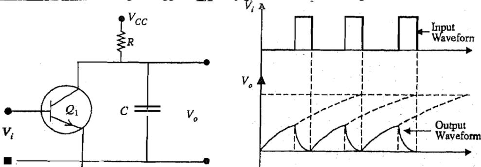
Fig.13.5 : Simple sawtooth generator and associated waveforms.
