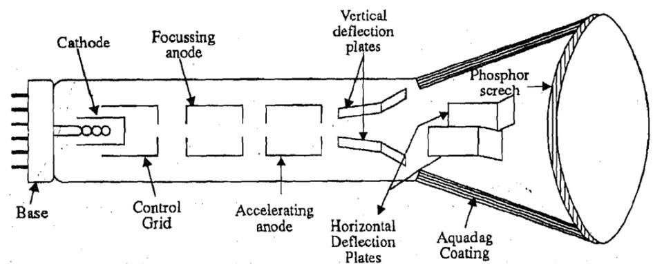
Fig.13.2 : Cathode ray tube with major components identified.
