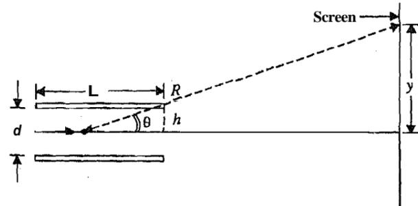
Fig.13.3 : Deflection of electron beam in CRT.
