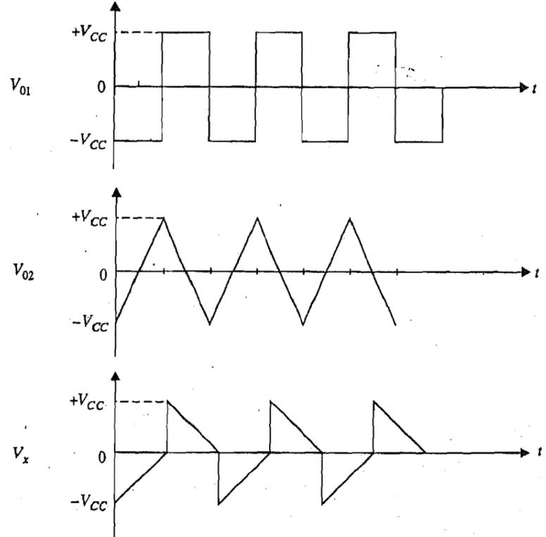
Fig.13.11 : Output waveforms for function generator.
