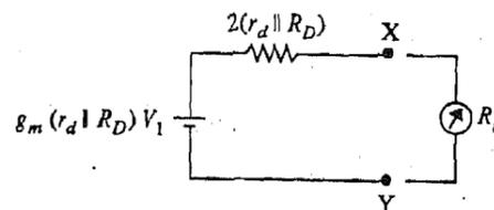
**Fig.13.16 : Equivalent circuit of EVM.**
