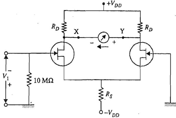
Fig.13.14 : The difference amplifier type EVM.
