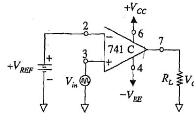
Fig.7.11: Comparator or voltage level detector.
