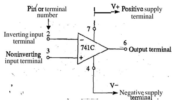
Fig.7.1: Circuit symbol for an op amp.
