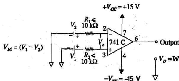
**Fig.7.6: Measuring input offset voltage.**
