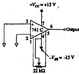
Fig.7.7: Adjusting output offset voltage.
