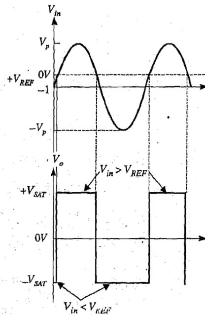
Fig.7.12: Output waveform of the comparator with  $+V_{REF}$
