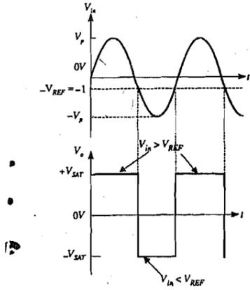
Fig.7.13: Output waveform of the comparator with  $-V_{REF}$ .
