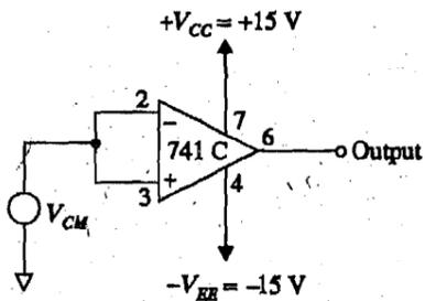
Fig.7.8: Common mode connections.
