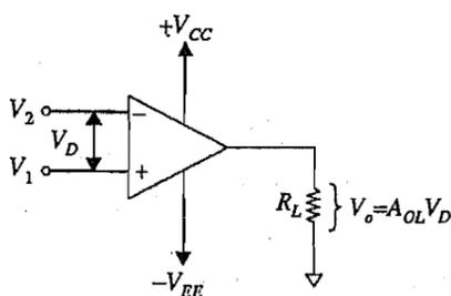
Fig.7.5: Output voltage depends on the input difference voltage.
