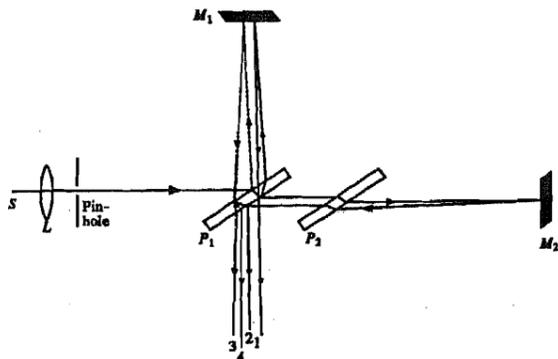
Fig. 7.8: Adjustment of Michelson Interferometer.
