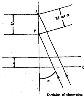
Fig. 7.3: Looking off-axis into the Michelson Interferometer.
