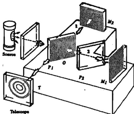
Fig. 7.1: Michelson Interferometer.
