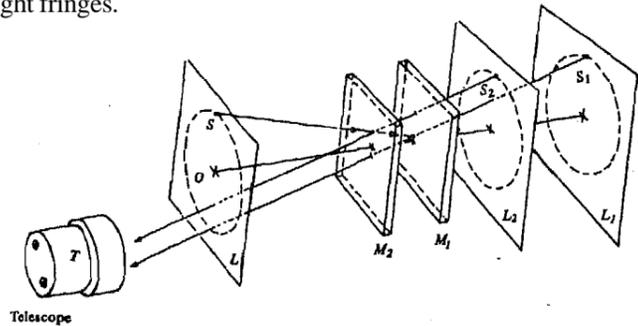
Fig. 7.2: A conceptual rearrangement of the Michelson Interferometer.
