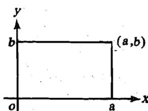
Fig. 6.2: A rectangular membrane fixed at edges
