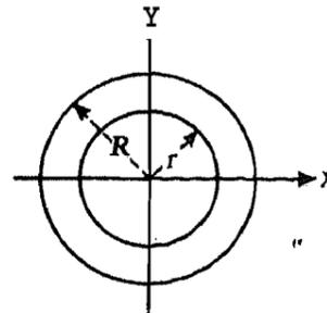
Fig. 6.3 : A circular membrane fixed at the perimeter
