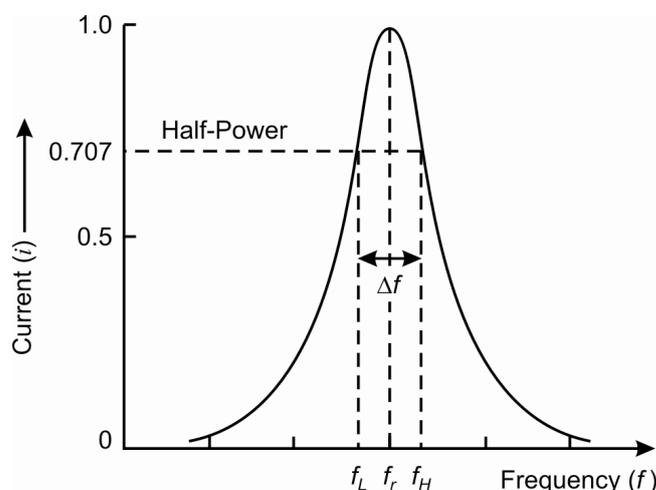
Fig. 8.3: Resonance curve for a series- $LCR$  circuit.  $f_r$  and  $\Delta f (= f_H - f_L)$  respectively denote resonance frequency and bandwidth.  $f_H$  and  $f_L$  are the higher and lower frequencies respectively of the bandwidth.
