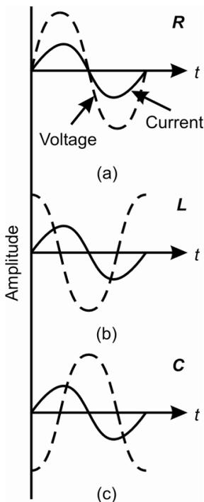
Fig. 8.1: Phase responses of a)  $R$ ; b)  $L$ ; and c)  $C$ , respectively
