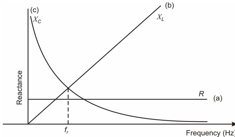
Fig. 8.2: Frequency dependence of reactance for a)  $R$ ; b)  $L$ ; and c)  $C$
