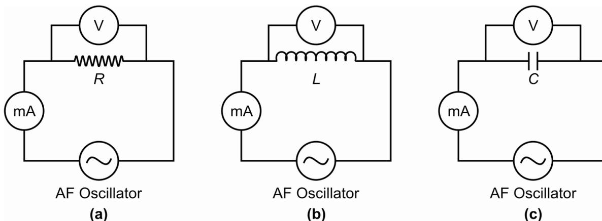
Fig. 8.5: Circuit diagram for studying frequency responses of a)  $R$ ; b)  $L$ ; and c)  $C$
