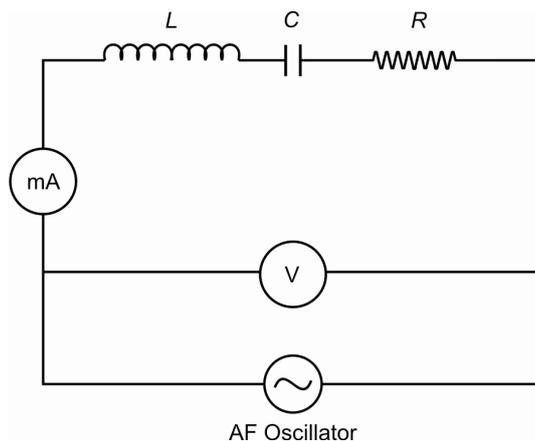
**Fig. 8.6: Circuit diagram for studying the frequency response of a series-LCR circuit**
