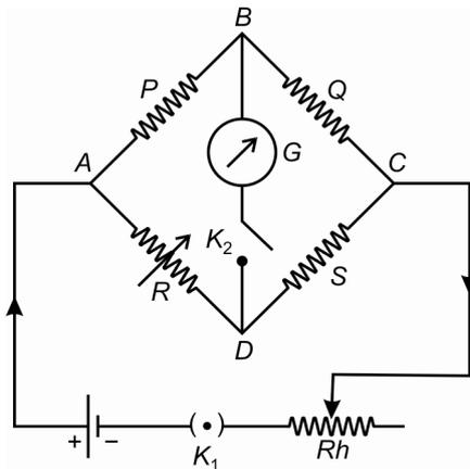
Fig.6.1: Circuit diagram of Wheatstone's bridge
