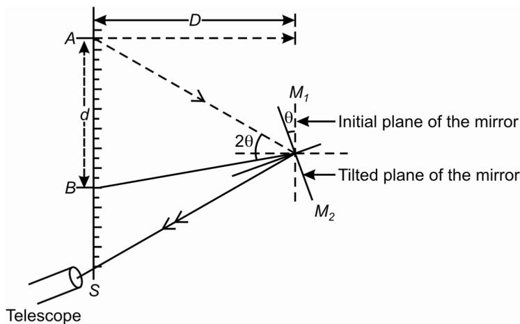
Fig.5.10: Illustrating the principle of optical lever
