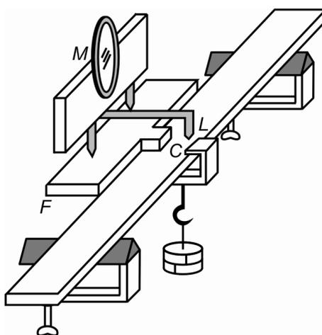
**Fig.5.9: Experimental arrangement for measuring depression of a beam using a telescope and an optical lever**
