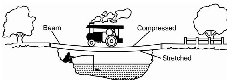
**Fig.5.1: A railway engine moving over a railway bridge produces depression in the beam**
