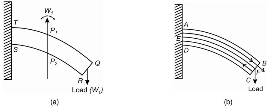
Fig.5.3: a) When a cantilever is loaded, it bends; and b) filaments in the interior of a cantilever under the action of a bending couple
