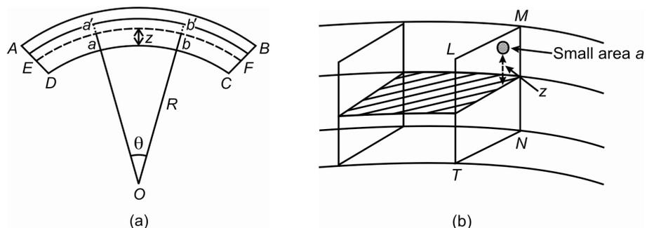
Fig.5.5: a) A small portion of the beam in strained condition; and b)  $LMNT$  is cross-section of the beam perpendicular to its length and the plane of bending.
