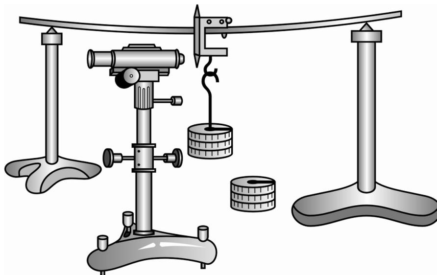
Fig.5.7: Experimental arrangement for measuring depression of the beam using a microscope
