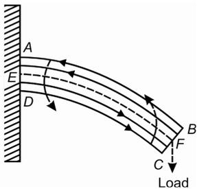
Fig.5.4: The moments of forces about the neutral axis indicated by dotted arrows oppose bending
