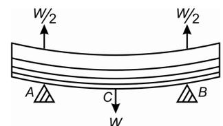
Fig.5.2: A beam supported near the two ends and loaded at the centre
