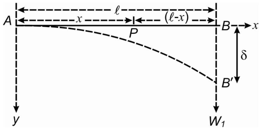
Fig.5.6: A cantilever of length  $\ell$  loaded at the free end
