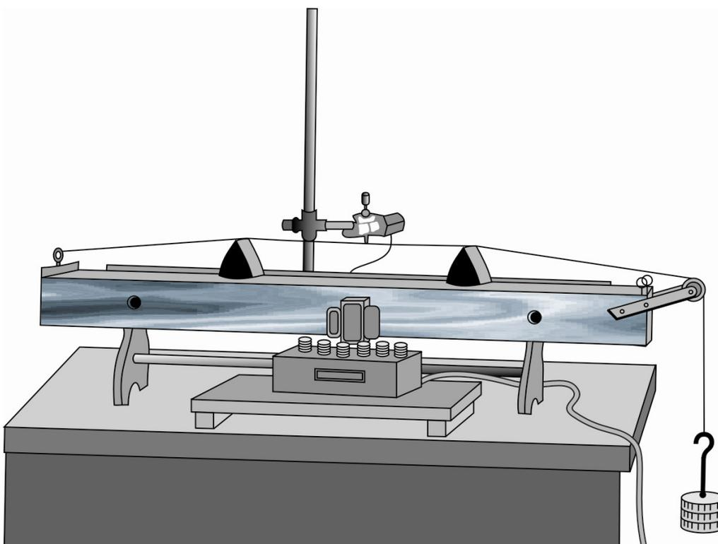
**Fig.4.3: Experimental arrangement for generating transverse stationary waves in a sonometer wire using an electromagnet**
