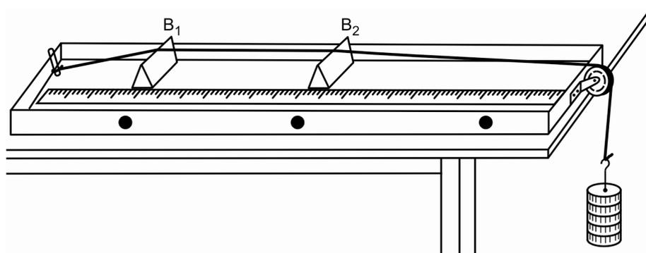
Fig.4.1: Stationary waves in a stretched string of a sonometer
