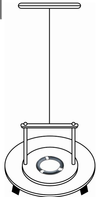
Fig.2.4: A torsional pendulum
