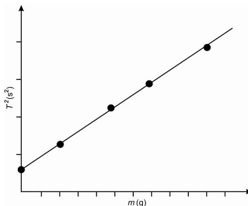
**Fig.2.3: Expected plot of  $T^2$  versus  $m$**
