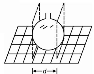
**Fig.1.3b: Determination of diameter of bob using graph paper**
