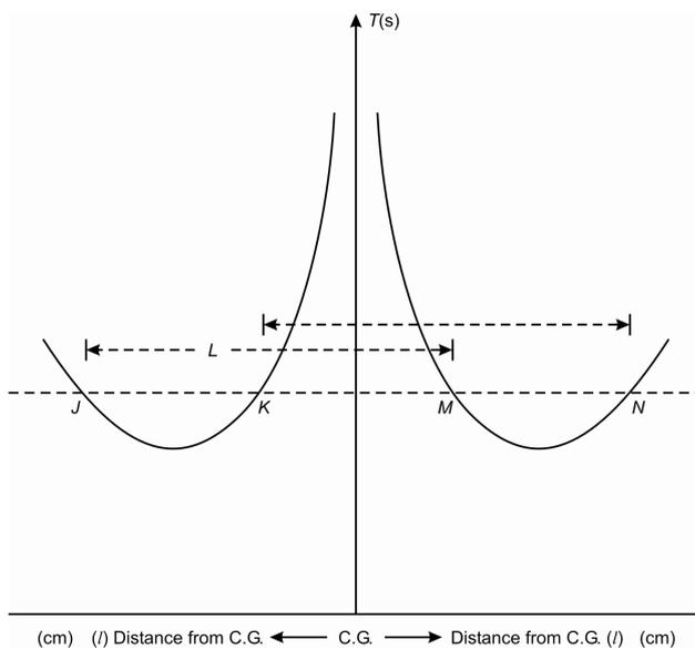
**Fig.1.6: Plot of time period with distance of point of suspension from C. G.**
