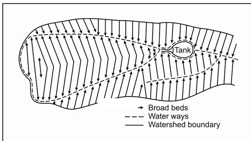
**Fig.11.5: Layout of beds and collection system for soil and water conservation purposes.**
