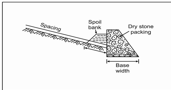
Fig.11.4: Stone terrace as seen in cross section
