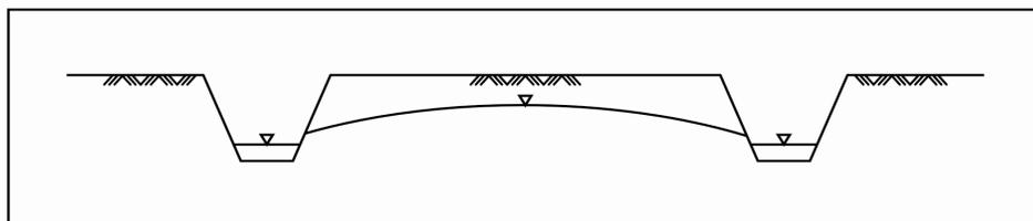
**Fig.11.6: Deep drains of subsurface drainage and water table control.**
