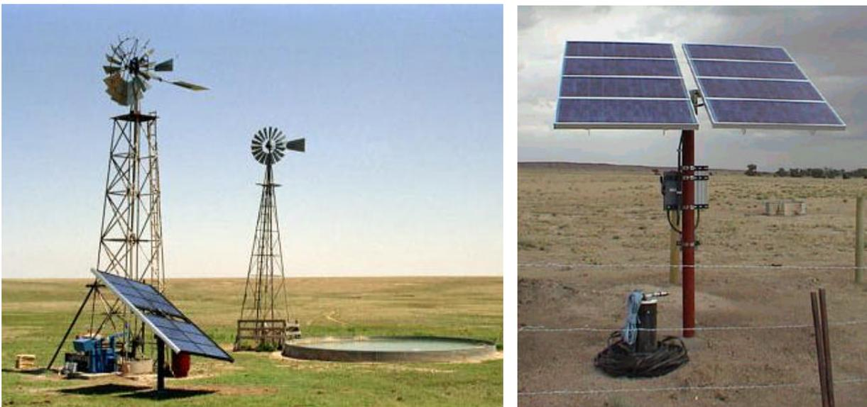
Fig.9.11: Solar water pumps
