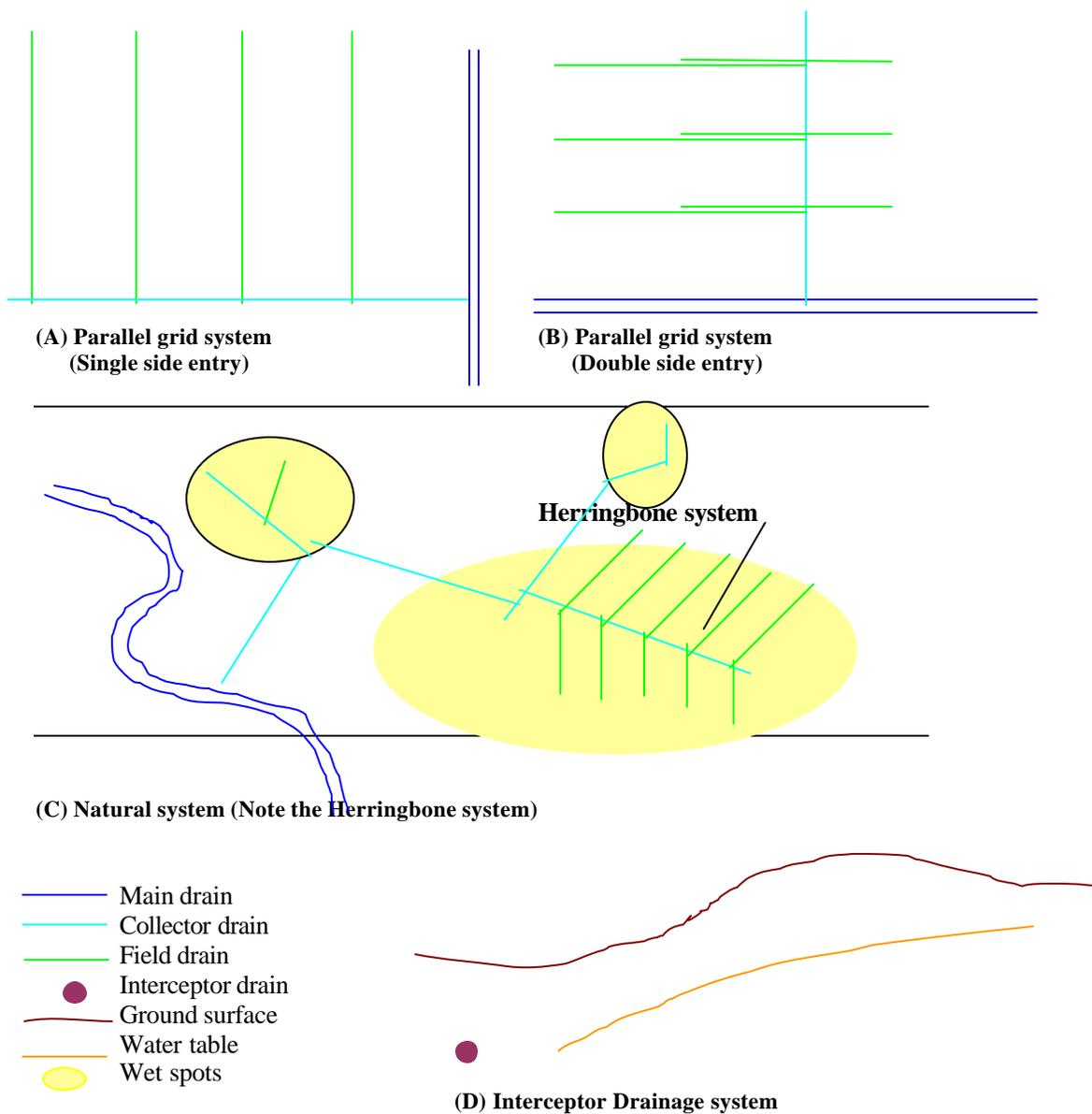
Fig.7.4: Standard layouts for drainage systems
