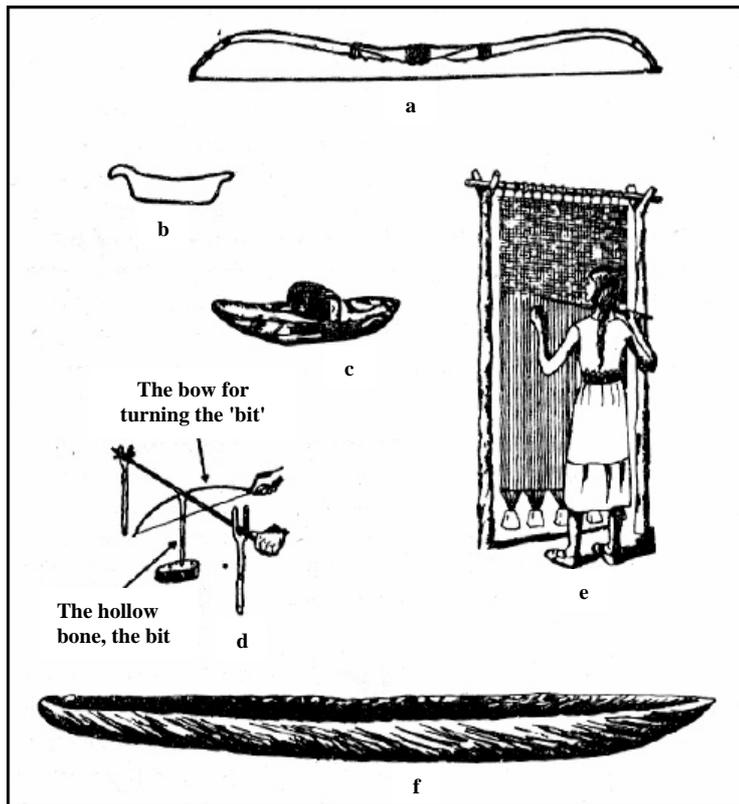
**Fig.1.3: Implements used towards the end of the Stone Age: a) composite bow; b) skin boat, outline from Norway; c) grain milling stone; d) bow drill for boring stone; e) weaving loom, reconstructed according to available remains and descriptions; f) boat made out of a tree trunk.**
