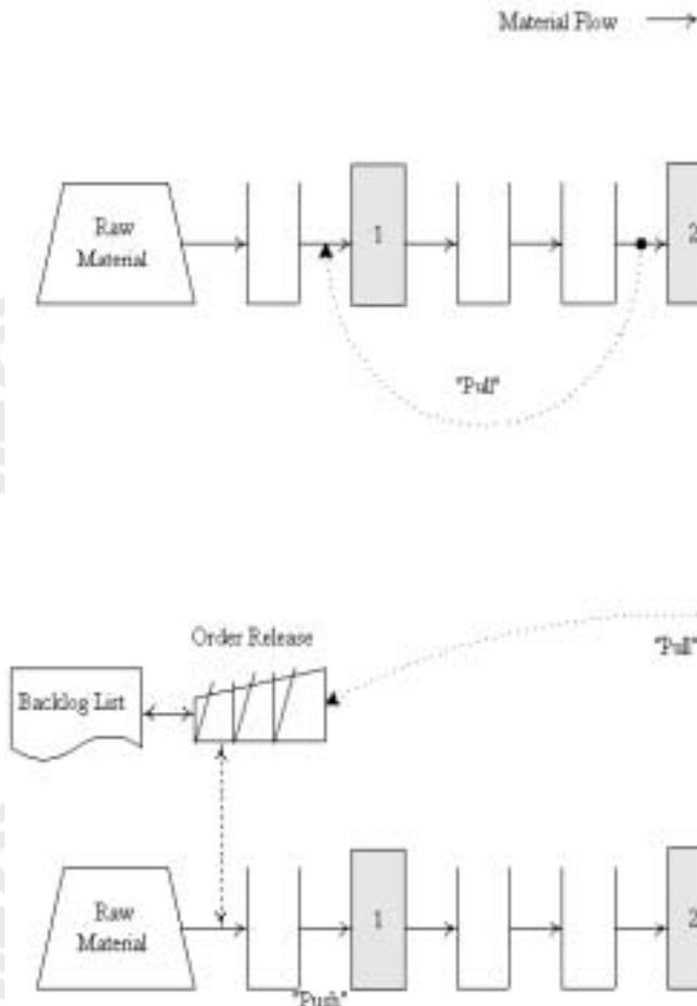
Figure 11.3: Comparison of Kanban and CONWIP Systems
