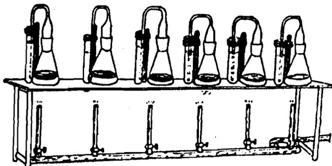
Set of Flasks Used for Reduction of Tin Salts
