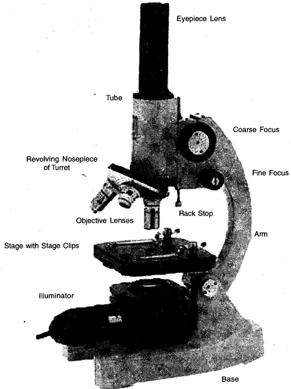
Fig. 10.1 Compound Microscope
