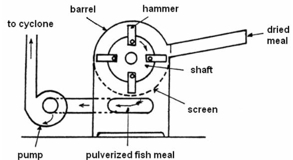
Fig.2.4: Hammer mill
