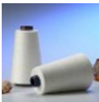
Fig. 9.10: Chitosan fibre yarn
