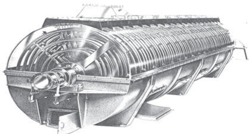
Fig. 1.9: Coil type indirect steam drier
