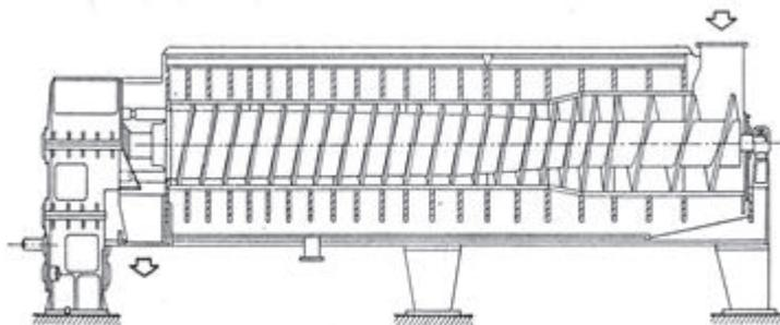
Fig. 1.6: Single screw press
