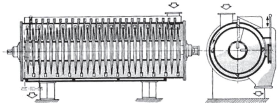
Fig. 1.8: Disc type indirect steam drier
