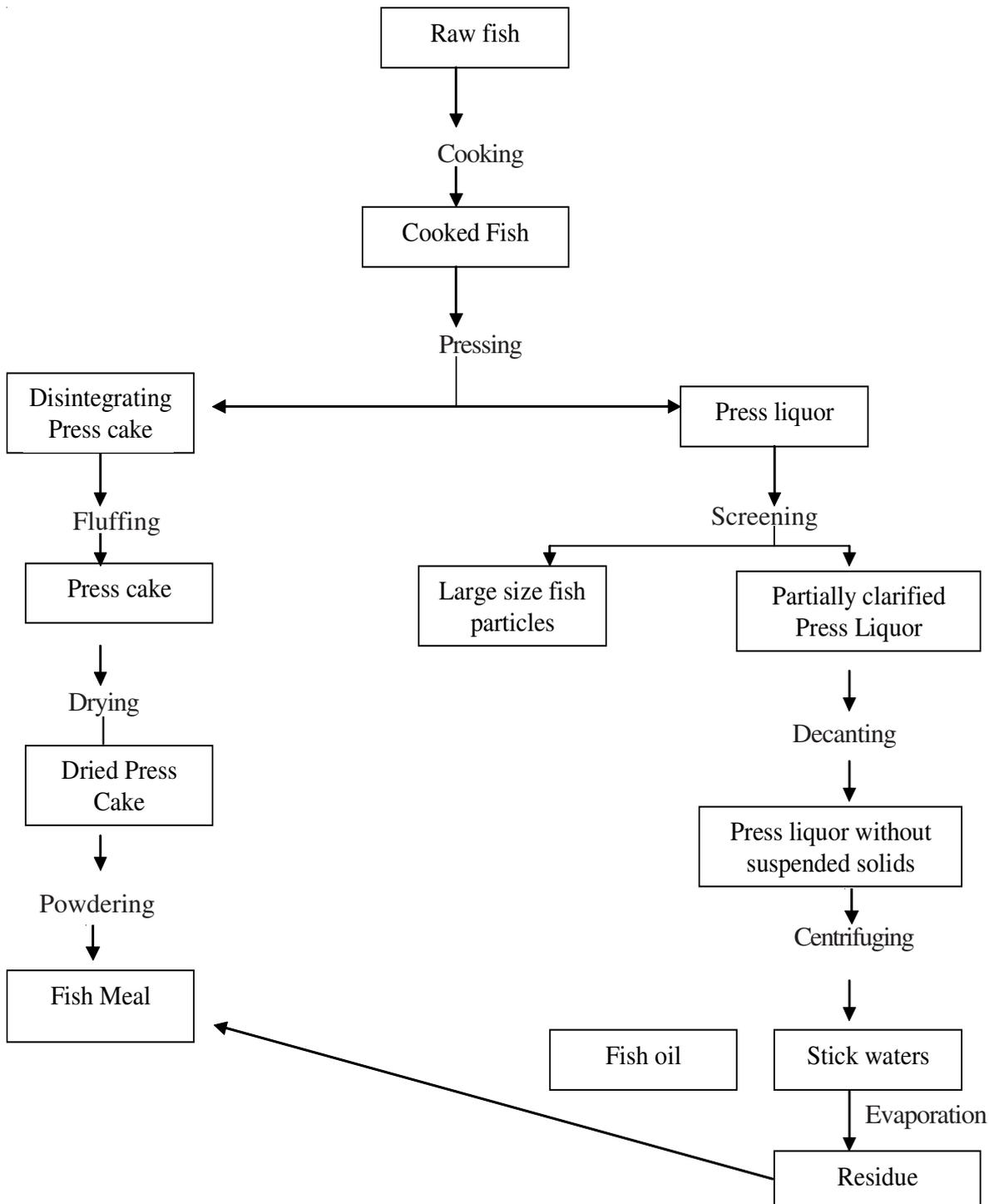
Fig. 1.3: Wet Reduction Method for Fish Meal and Oil Manufacture
