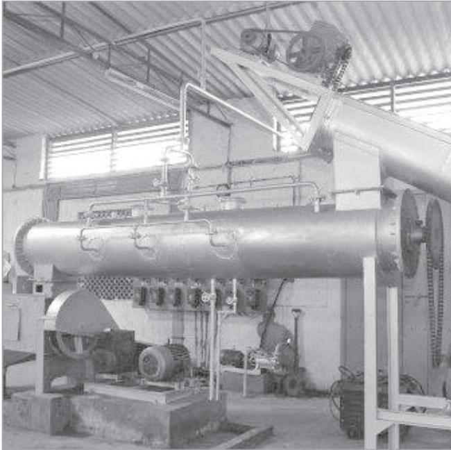
Fig. 1.5: Cooker for cooking fish in fish meal plant
