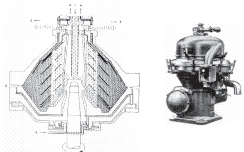
**Fig. 1.12: Conical disc type centrifuge**
