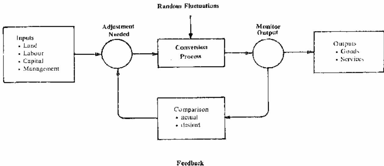
Figure I describe a generalised concept of production system. It takes resource inputs and processes them to produce useful outputs in the form of goods or services.
