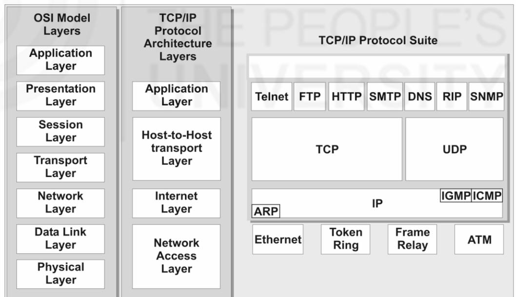
Fig. 15.8: Comparison of OSI and TCP/IP Models
