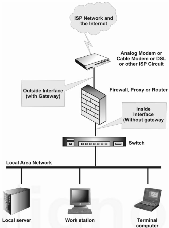
Fig. 15.1: Typical configuration showing Internet access via ISP
