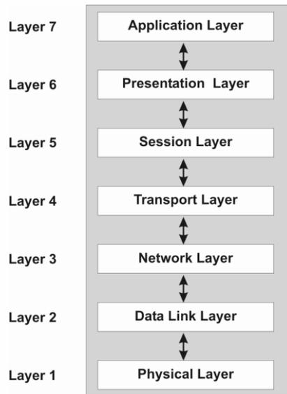
Fig. 15.3: Network architecture based on the OSI model
