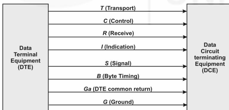
Fig. 15.4: Signal lines used in X.21
