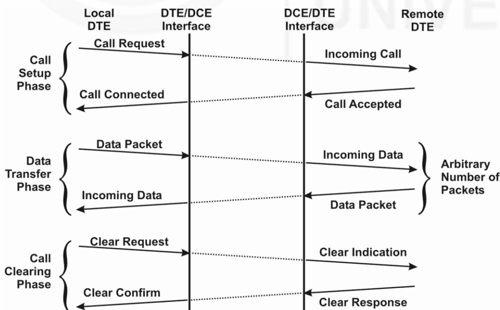
Fig. 15.6: The three phases of an X.25 connection
