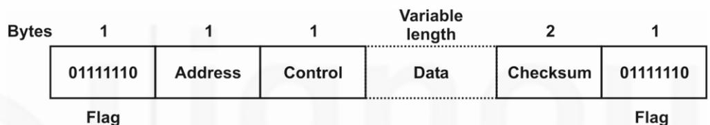
**Fig. 15.5: Frame format for bit-oriented protocols**
