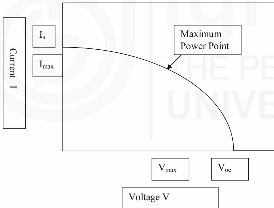
Figure 4.4 : Voltage-current Characteristics of a Solar Cell
