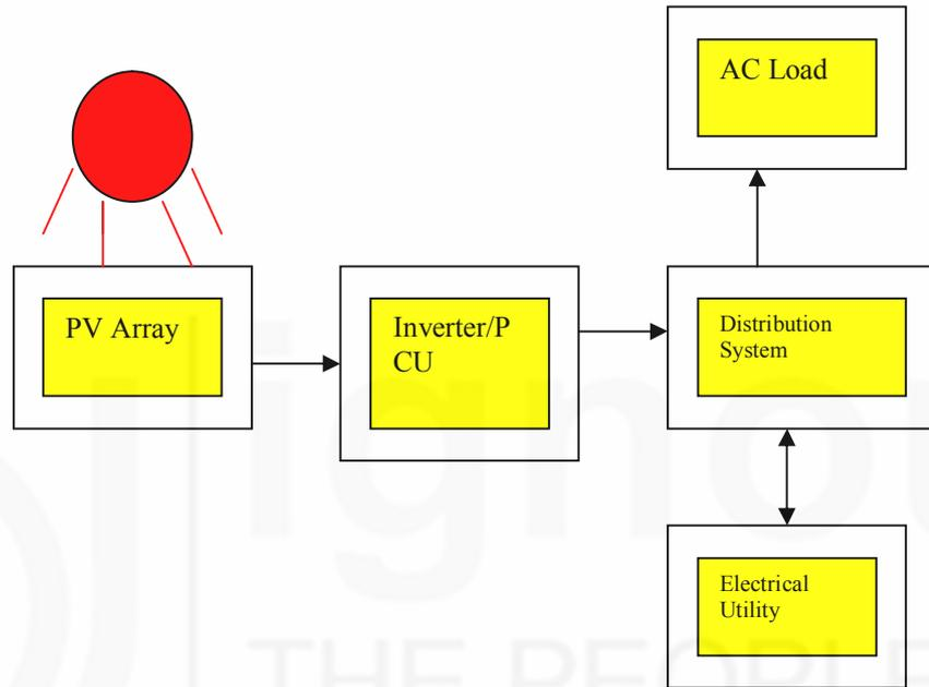
Figure 4.6 : A Schematic Diagram of Grid-connected PV System
