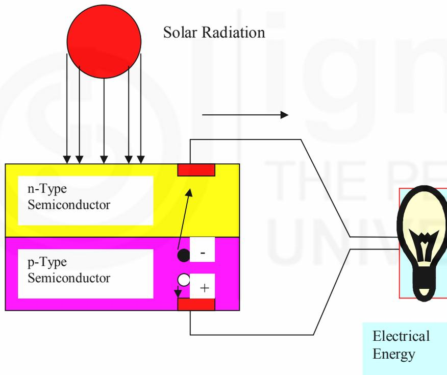
**Figure 2.1 : Photovoltaic Effect**
