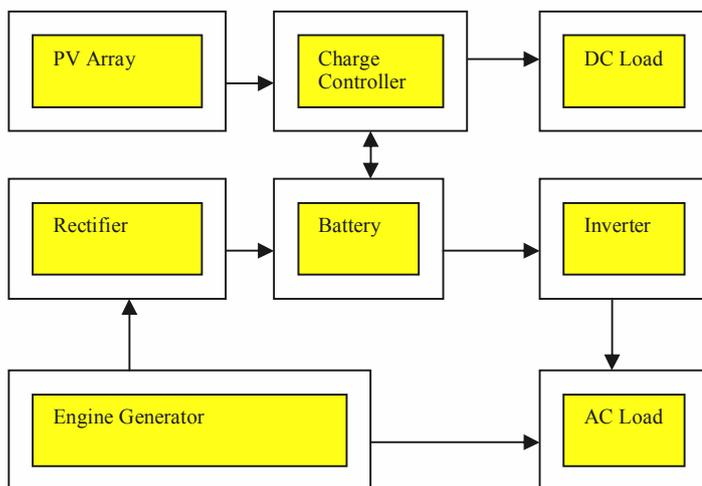
Figure 4.9 : Diagram of Photovoltaic Hybrid System
