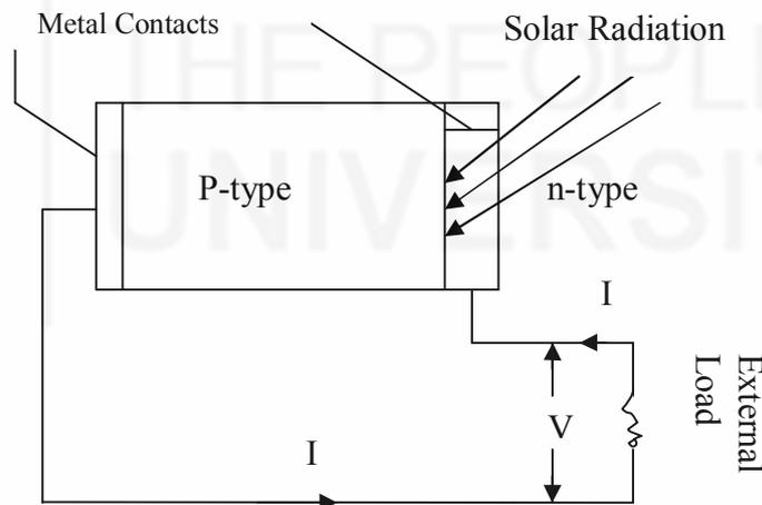
**Figure 4.2 : Operation of a Photovoltaic Junction**
