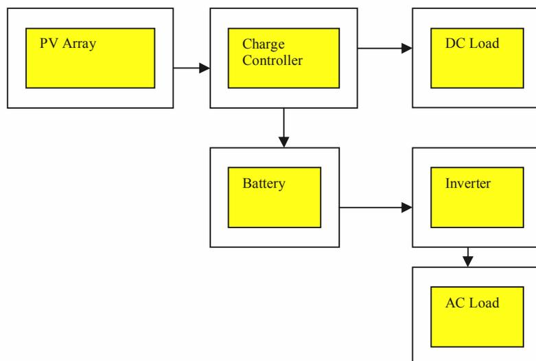
Figure 4.8 : Diagram of Stand-alone PV System with Battery Storage Powering DC and AC Loads
