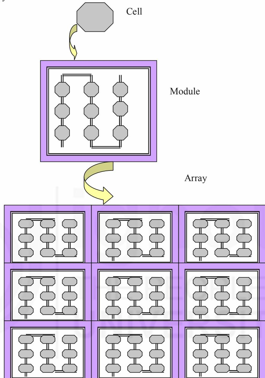
Figure 4.5 : PV Cells, Modules and Arrays
