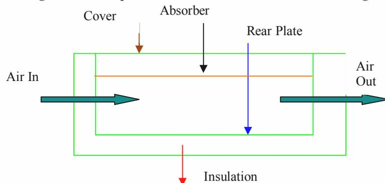
**Figure 4.3 : Nonporous Type Solar Air Heater with Glazing**
