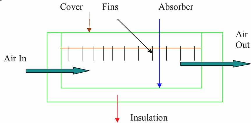
**Figure 4.5 : Nonporous Type Solar Air Heater with Fins**
