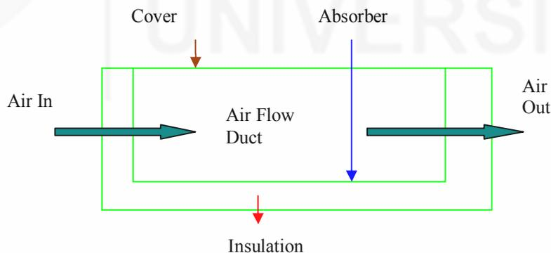
**Figure 4.2 : Nonporous Type Solar Air Heater with Glazing**
