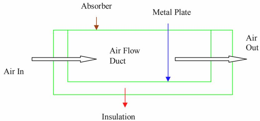
**Figure 4.1 : Nonporous Type Solar Air Heater**
