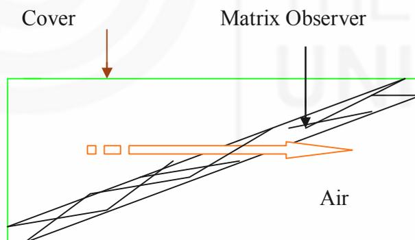
Figure 4.6 : Porous Type Solar Air Heater
