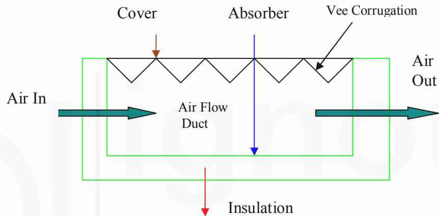
**Figure 4.4 : Nonporous Type Solar Air Heater with Vee Corrugation**
