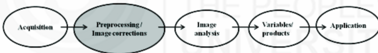
Fig. 11.1: Chain of broad steps in remote sensing data processing
