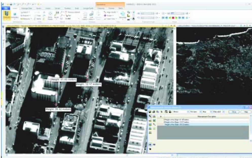
**Fig. 7.2:** A snapshot of the ERDAS Imagine software showing measurement of height of image features (source: [www.erdas.com/products/ERDASIMAGINE/ERDASIMAGINE/Details.aspx](http://www.erdas.com/products/ERDASIMAGINE/ERDASIMAGINE/Details.aspx))
