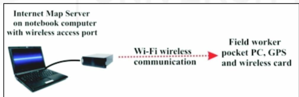
Fig. 2.11: Illustration of the concept of Mobile GIS (source: [www.map.sdsu.edu/fireweb/mobileGIS.htm](http://www.map.sdsu.edu/fireweb/mobileGIS.htm))
