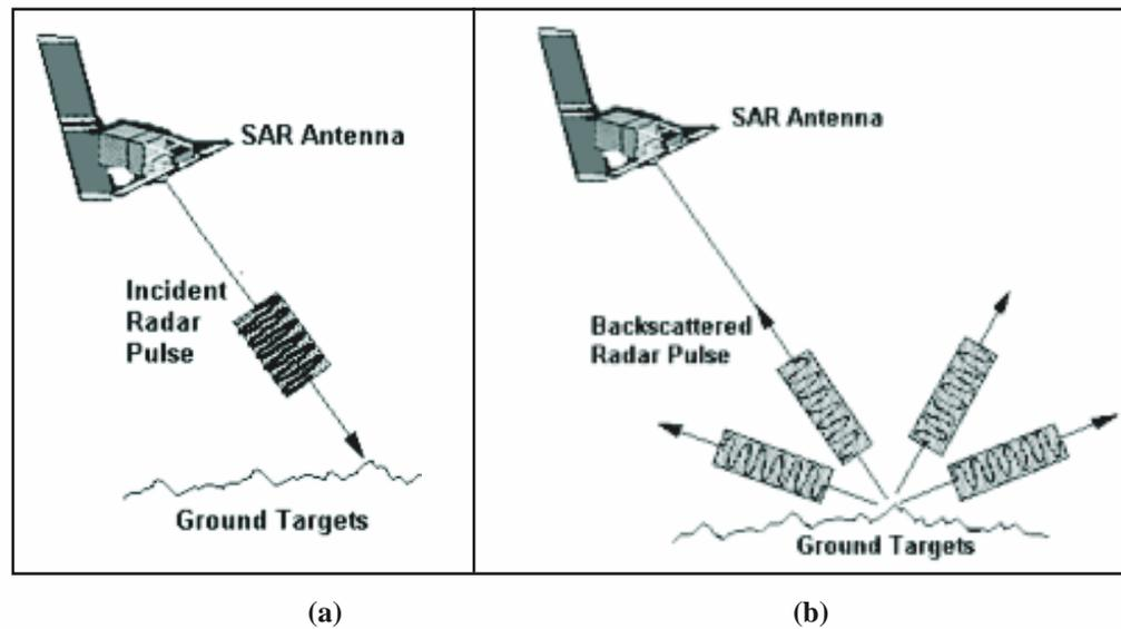
Fig. 2.7: Illustration showing the concept of SAR imaging; a) A radar pulse is transmitted from the antenna to the ground, b) The radar pulse is scattered by the ground targets back to the antenna
