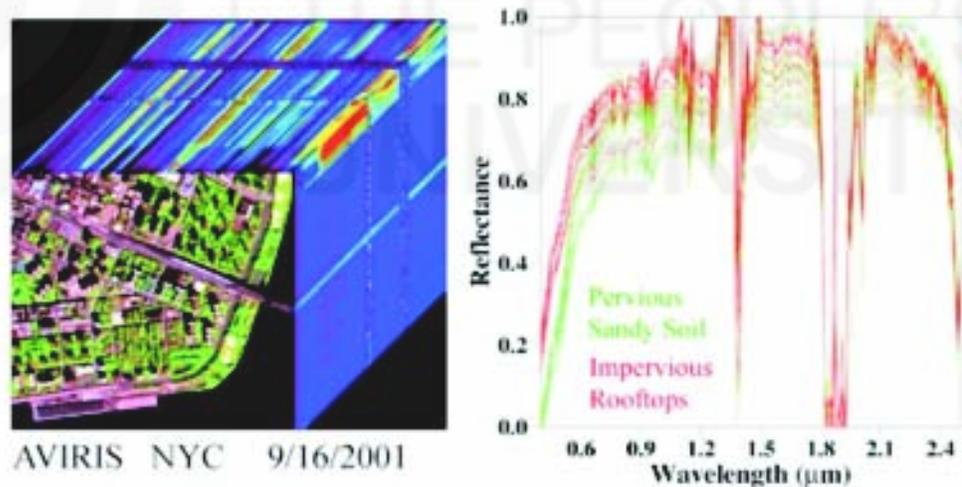
**Fig. 2.5:** Image data cube and spectral response pattern of different materials as obtained from a hyperspectral remote sensing image (source: [www.ldeo.columbia.edu/~small/Urban/UrbanHyperspectral.htm](http://www.ldeo.columbia.edu/~small/Urban/UrbanHyperspectral.htm))
