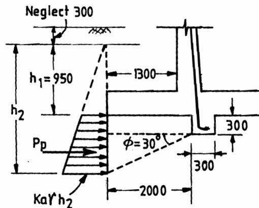
Figure 21.15 : Shear Key
