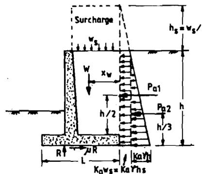
Figure 21.9 : Effect of Surcharge on a Level Backfill
