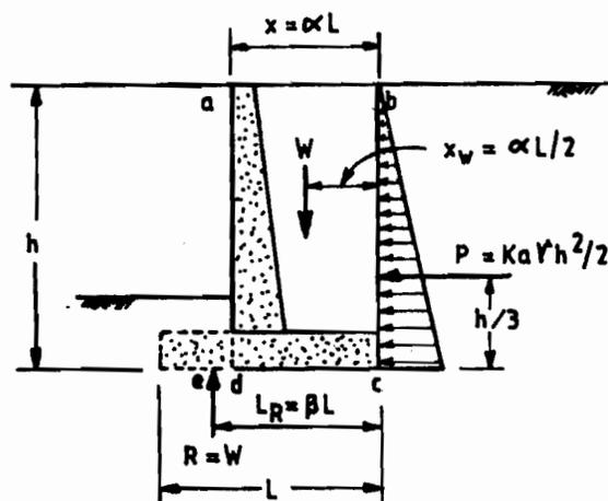
Figure 21.12 : Proportioning of Retaining Wall
