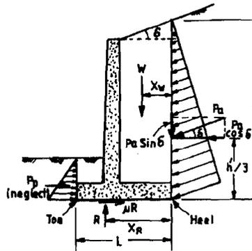
Figure 21.8 : Forces Acting on a Cantilever Retaining Wall
