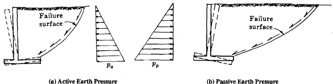
Figure 21.6 : Active and Passive Earth Pressures
