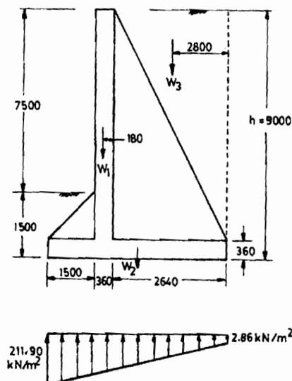
Figure 21.18 : Preliminary Dimensions of Counterfort Retaining Wall and Soil Pressure
