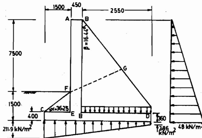
Figure 21.24 : Forces on the Counterfort Wall
