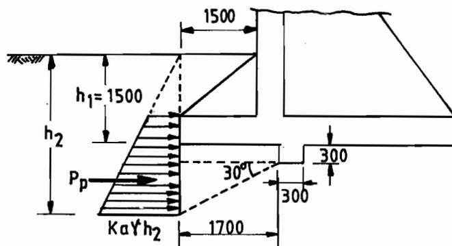
Figure 21.19 : Shear Key and Passive Pressure
