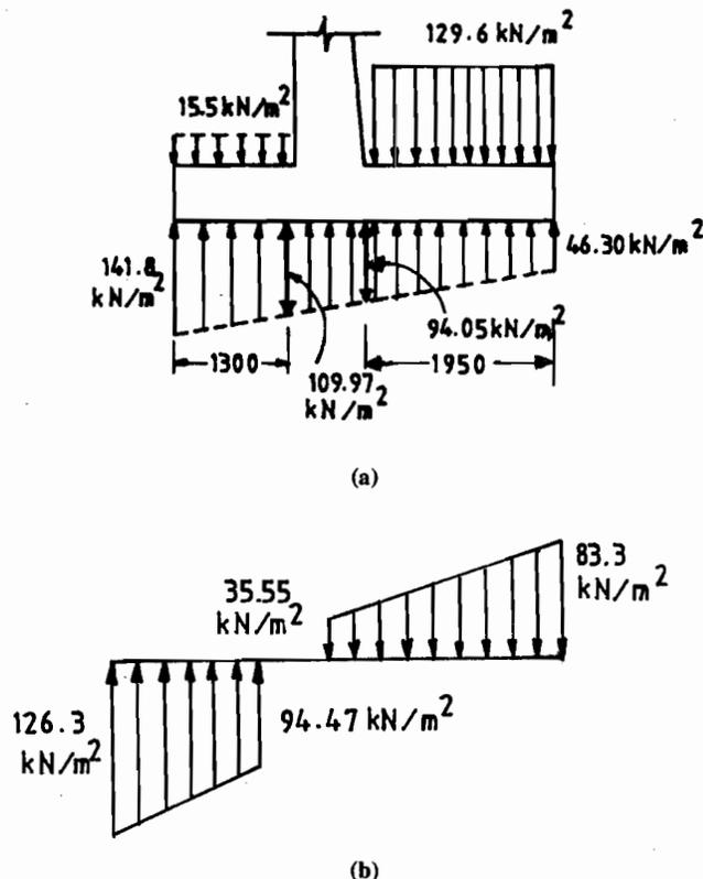
Figure 12.16 : Net Soil Pressure Acting on Base Slab
