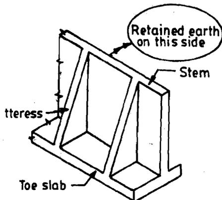
Figure 21.4 : Buttress wall
