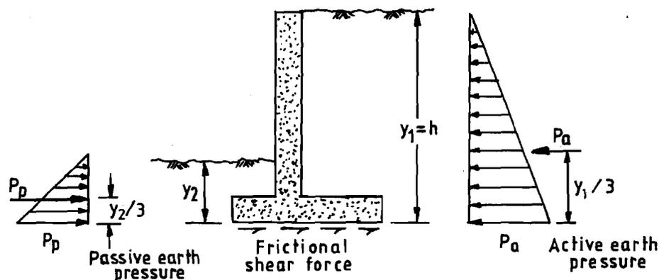
Figure 21.7 : Pressure Diagram
