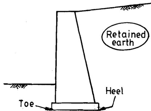
Figure 21.1 : Gravity Wall
