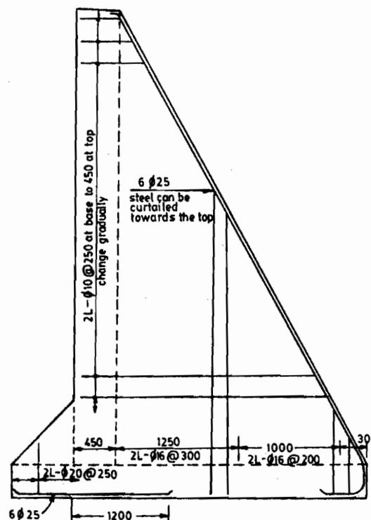
Figure 21.25 : Reinforcement in Counterforts (*Slab Reinforcement not shown*)
