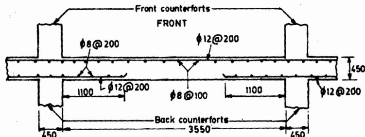
Figure 21.22 : Horizontal Section through Stem Slab Showing Reinforcement
