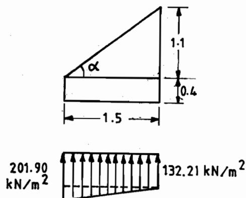
Net upward reaction at the end of toe
