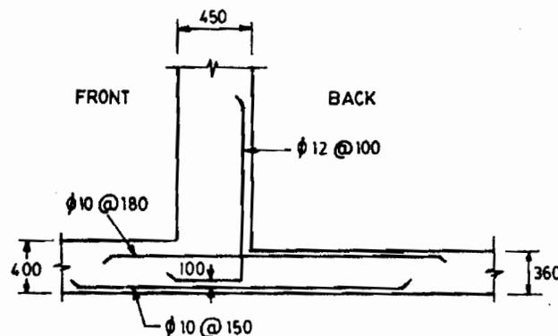
Figure 21.26 : Steel for Providing Fixidity Effect
