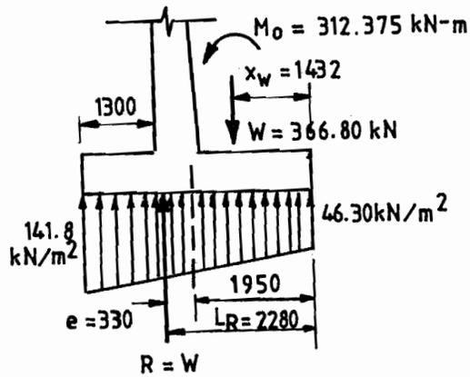
Figure 21.14 : Soil Pressure Distribution
