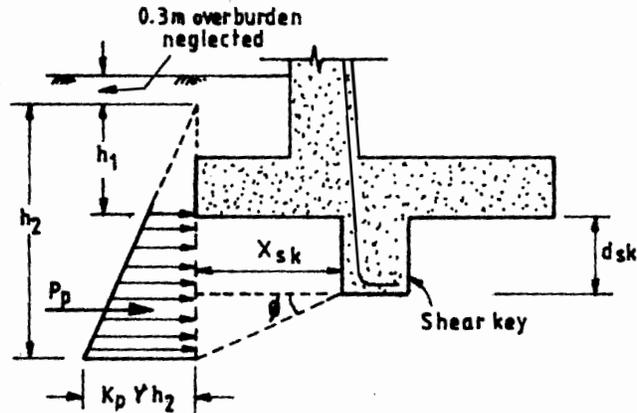
Figure 21.10 : Passive Resistance Due to Shear Key
