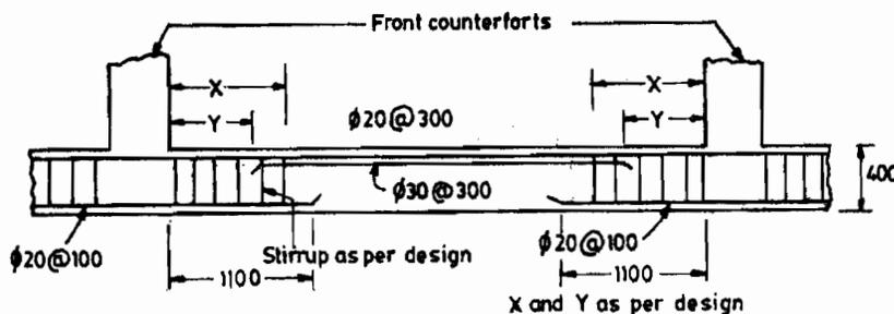
Figure 21.23 : Vertical Section of Toe Slab showing Reinforcement
