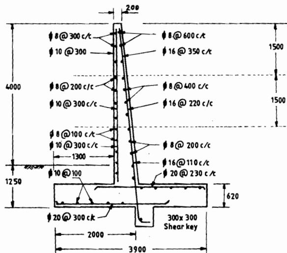
Figure 21.17 : Reinforcement Details of Cantilever Wall
