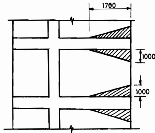
Figure 21.20 : Plan Showing Shear Stirrups Zone in Heel Slab
