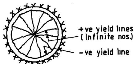
Figure 20.17 : Yield Line Pattern in a Circular Slab Carrying Uniformly Distributed Load
