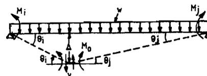
(c) Slab segments for virtual work method
