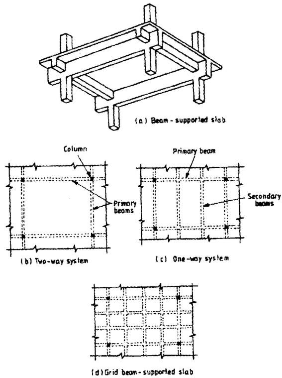
Figure 20.2 : Beam-supported Slab Systems
