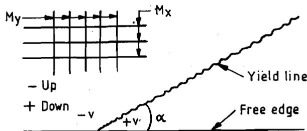
Figure 20.10 : Two-way Slab with a Free Edge
