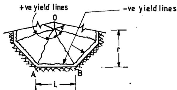
Figure 20.16 : Yield Line Pattern in a Polygonal Slab Carrying Uniformly Distributed Load
