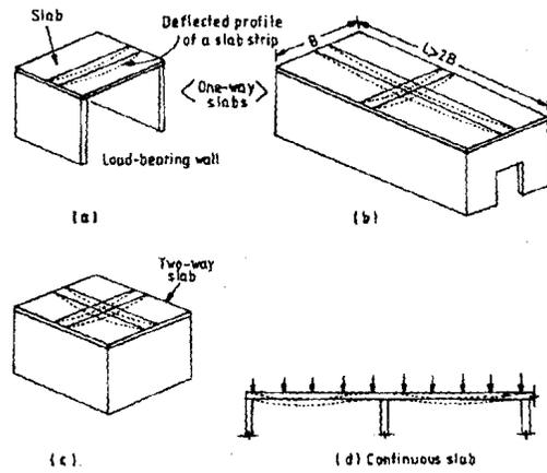
Figure 20.1 : Wall-supported Slab Systems
