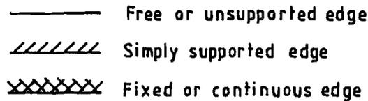
Figure 20.5 : Convention for Showing the Edges of Slabs
