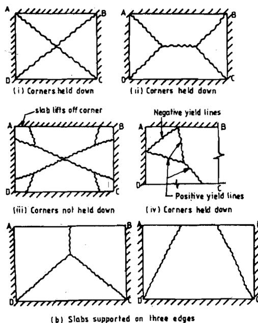
Figure 20.11 : Yield Patterns for Two-way Slabs
