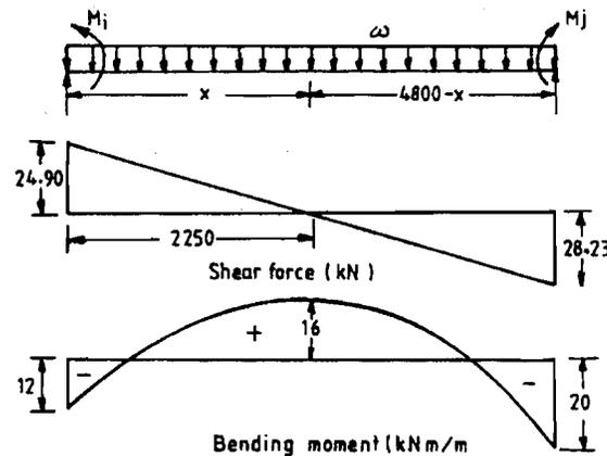
Figure 20.8 : Shear Force and Bending Moment Diagrams of One-way Continuous Slab
