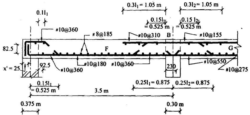
Figure 12.5 : Reinforcement Details of One Way Continuous Slab
