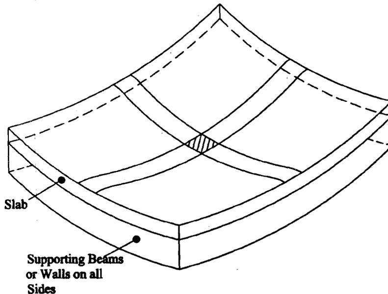
Figure 12.6 : Bending of Two Way Slab
