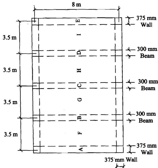
**Figure 12.4 : A Continuous One Way Slab**
