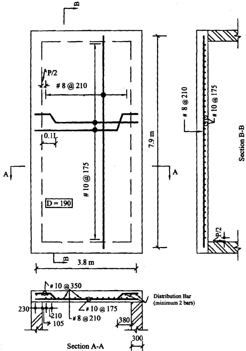
Figure 12.3 : Reinforcement Detailing of the Designed Slab
