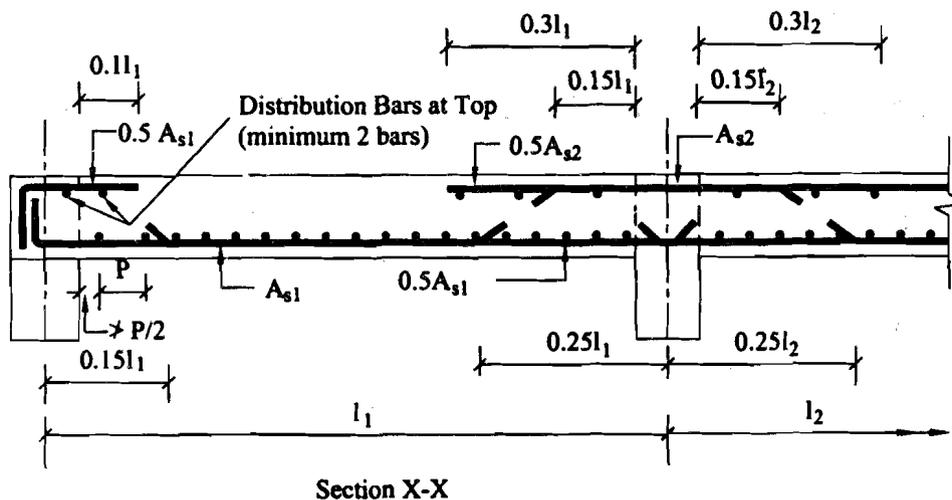
Figure 12.8 : Curtailment Rules for Two Way Slab
