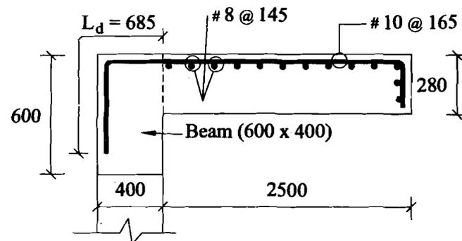
Figure 12.14 : Details of Reinforcement of Cantilever Slab Designed
