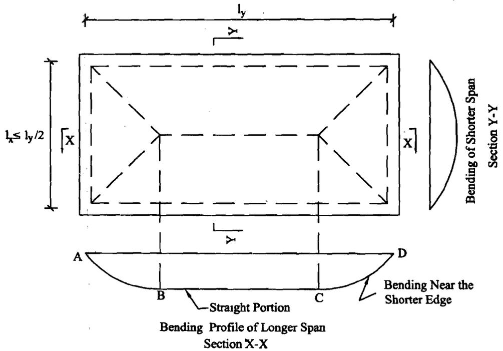
Figure 12.2 : Bending Profile of an One Way Slab Supported on all Edges
