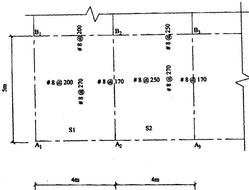
Figure 12.11 : Showing Reinforcement of the Designed Slab
