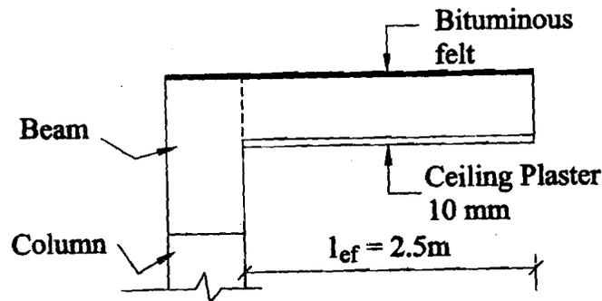
Figure 12.13 : A Cantilever Slab
