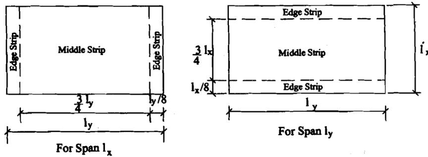
Figure 12.7 : Division of Slab into Middle and Edge Strips
