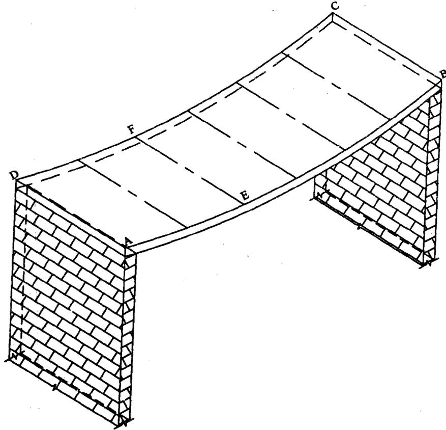
Figure 12.1 : Bending of One Way Slab Supported on Two Opposite Edges
