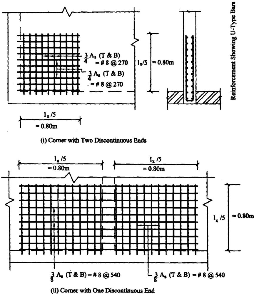
Figure 12.12 : Torsional Reinforcement in Slab
