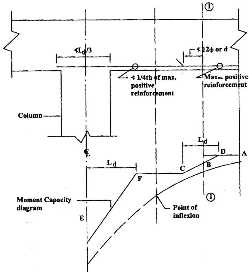
Figure 5.12 (b) : Curtailment of Positive Moment Reinforcement at Continuous Edge
