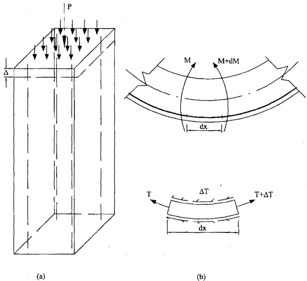
Figure 5.1 : Explaining the Effect of Proper Bond between Concrete and Reinforcement
