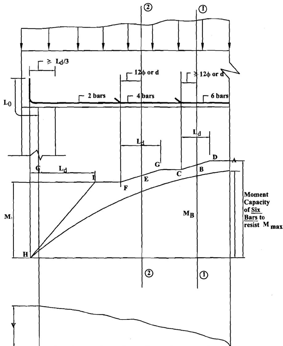
Figure 5.10 : Curtailment of Positive Reinforcement at Simple Support
