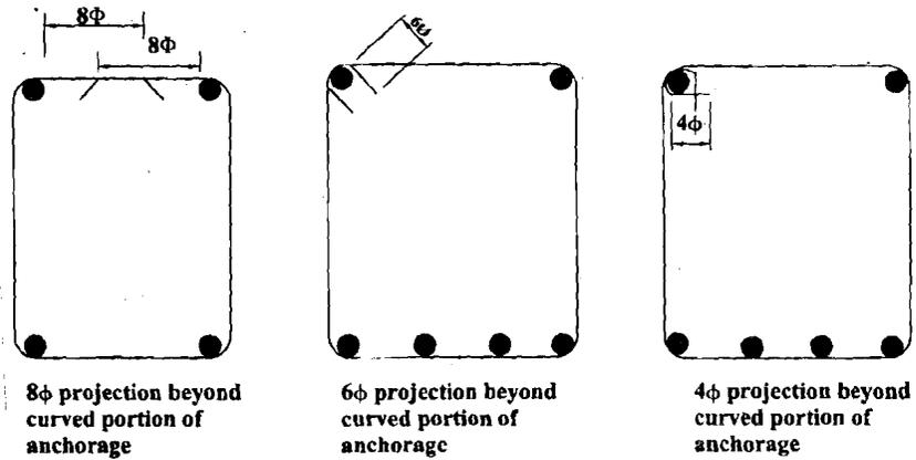
Figure 5.9 : Anchorages for Shear Reinforcements
