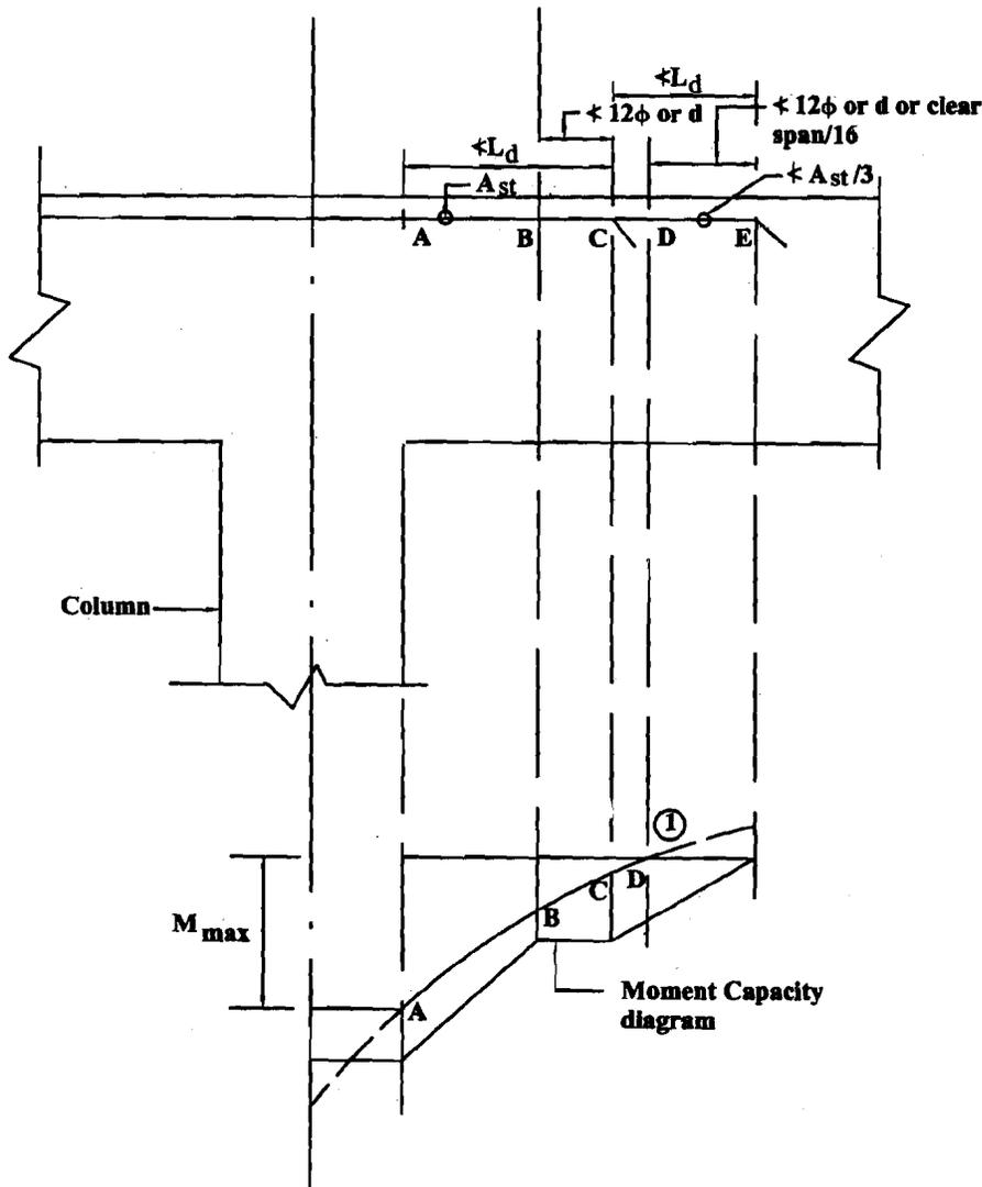
Figure 5.12 (a) : Curtailment of Negative Moment Reinforcement at Continuous Edge
