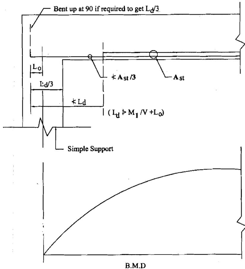
**Figure 5.5 : Tensile Development Length at Simple Support for Beams and Slabs**
