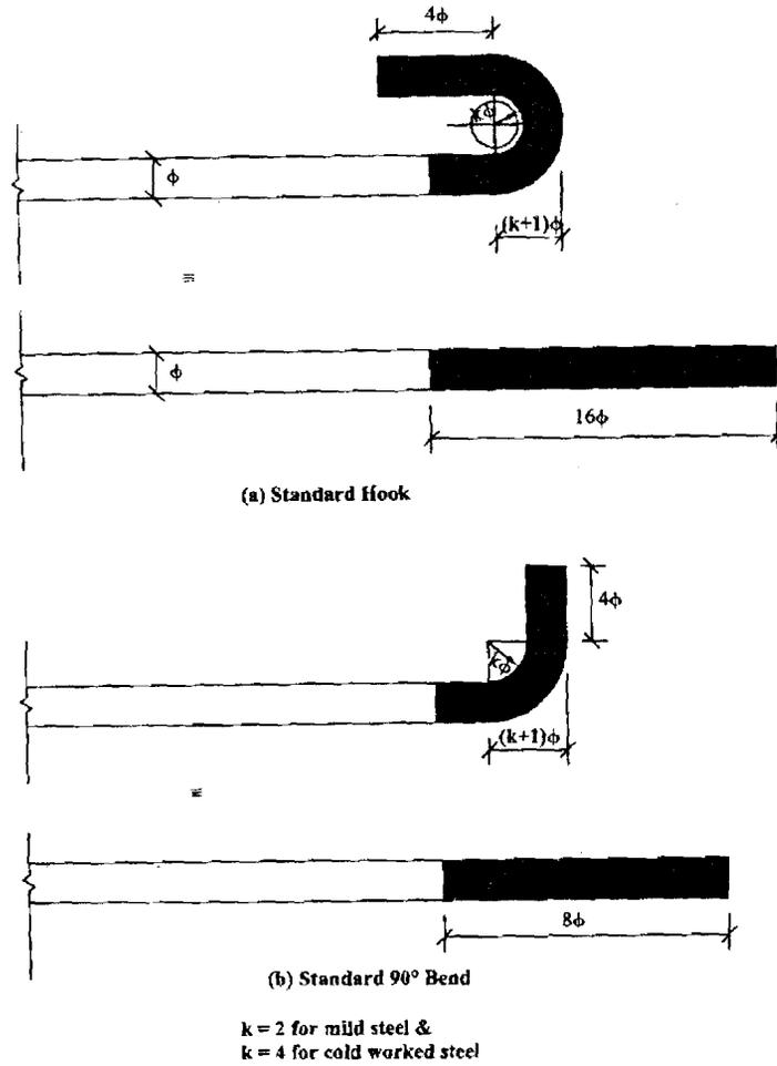
Figure 5.7 : Standard Hooks and Standard 90° Bend
