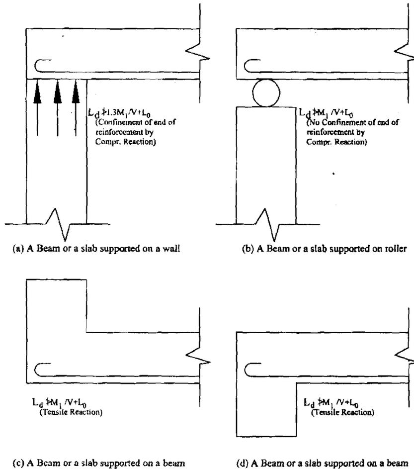
Figure 5.6 : Different Support Conditions for a Beam of a Slab
