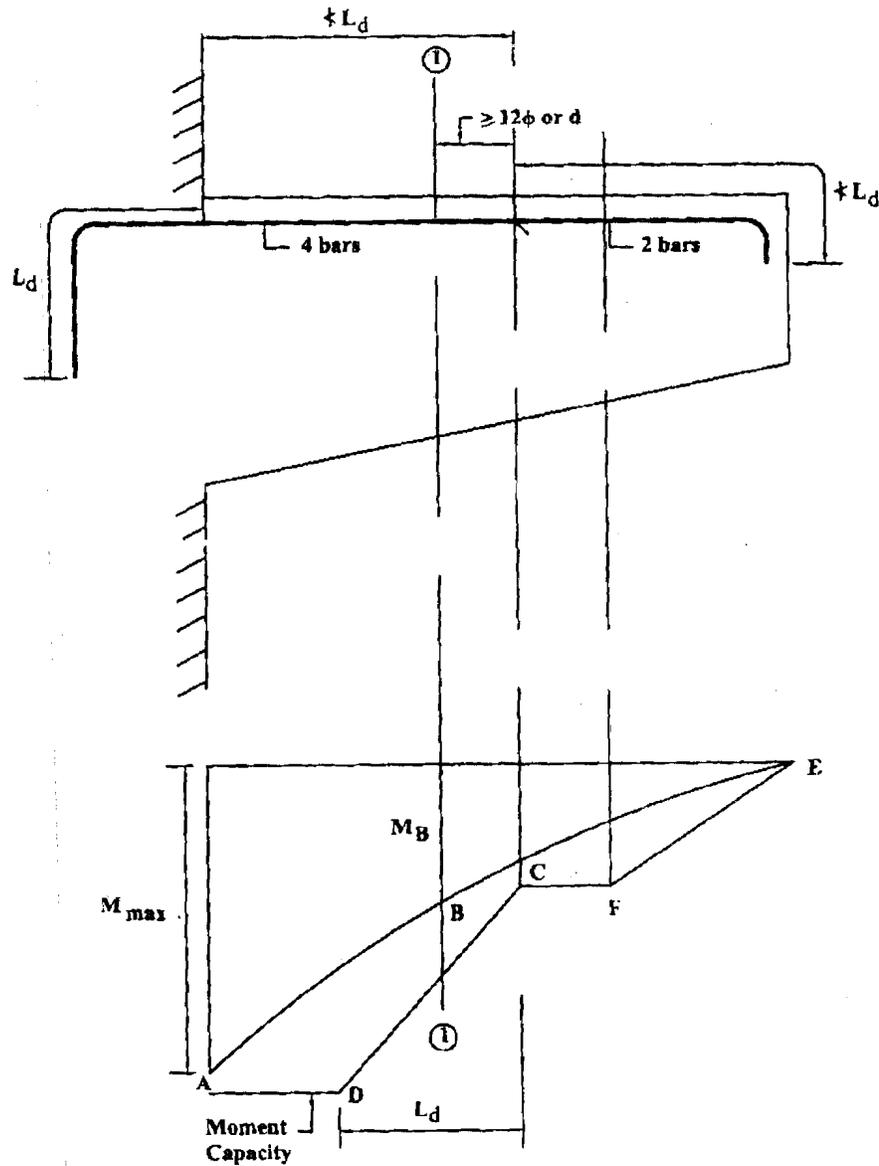
Figure 5.11 : Curtailment of Main Reinforcement of a Cantilever Beam
