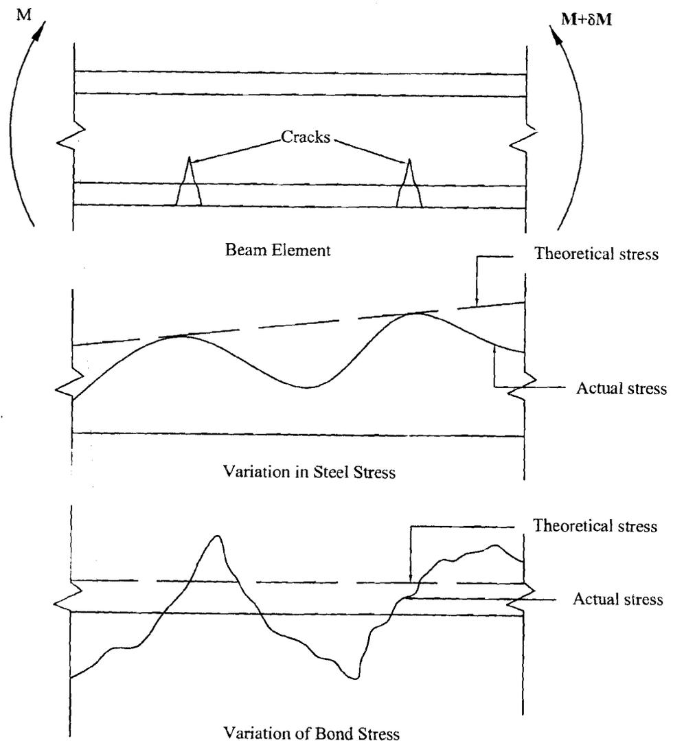
Figure 5.3 : Showing Variation between Actual Bond Stress and Theoretical Bond Stress
