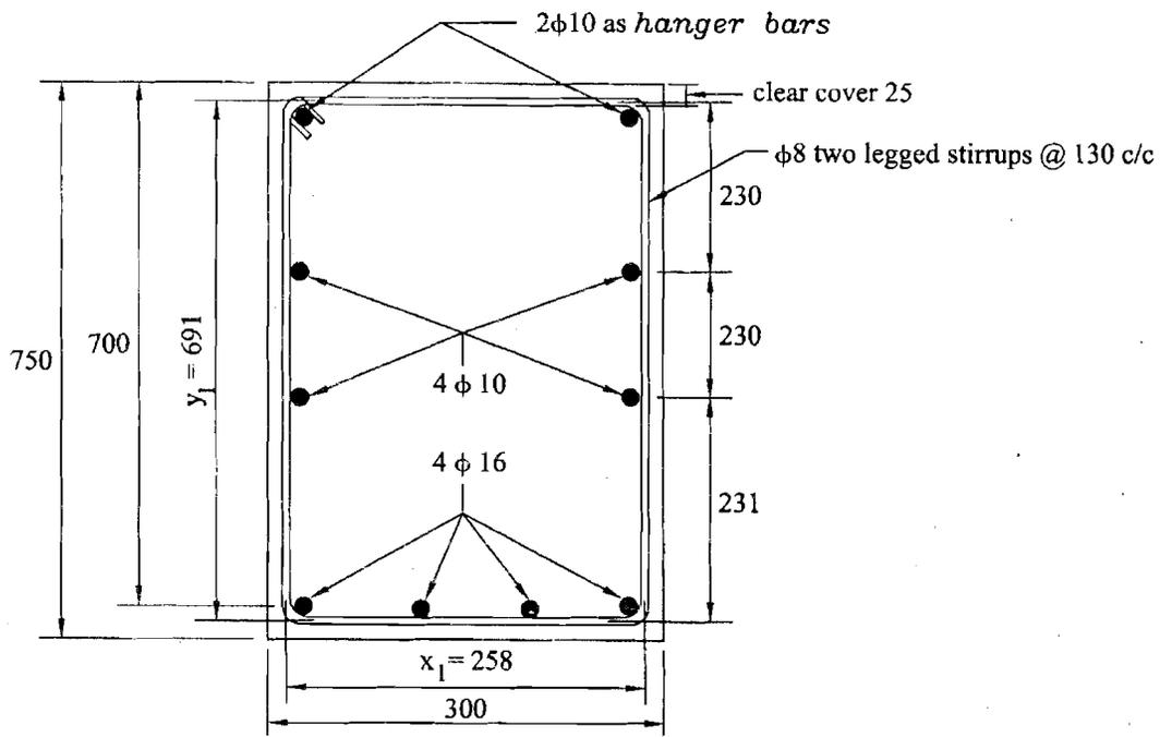
Figure 4.9 : Details of Reinforcement for Combined  $M_v$ ,  $V_v$ , and  $T_v$  having  $M_t > M_u$
