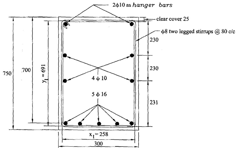
Figure 4.8 : Details of Reinforcement for Combined  $M_u$ ,  $V_u$ , and  $T_u$  having  $M_u < M_u$
