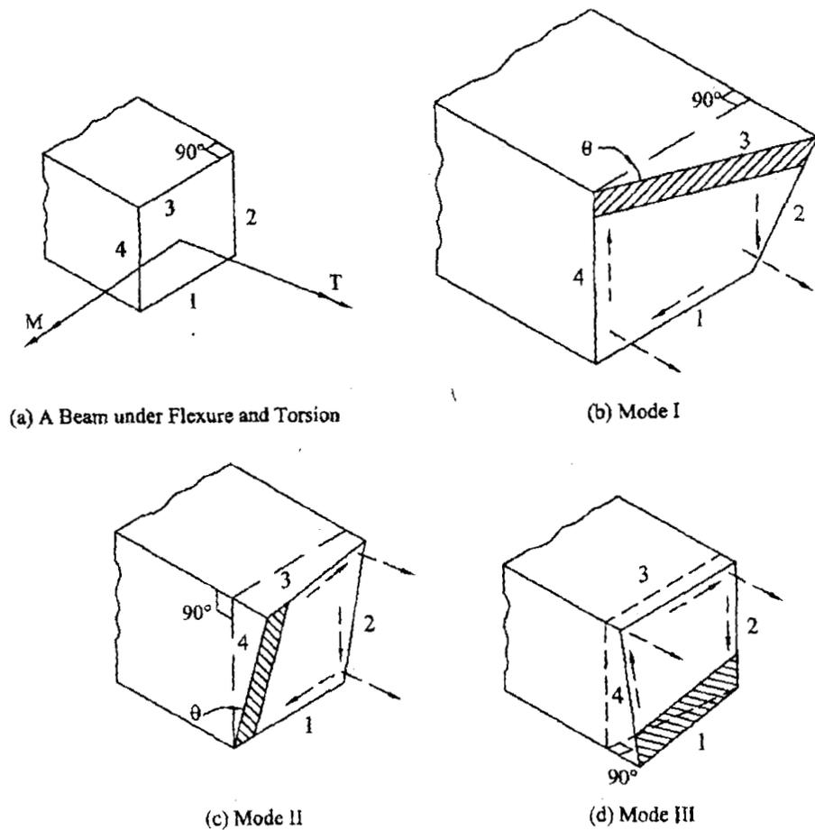
Figure 4.4 : Showing Different Modes under Combined Flexure & Torsion
