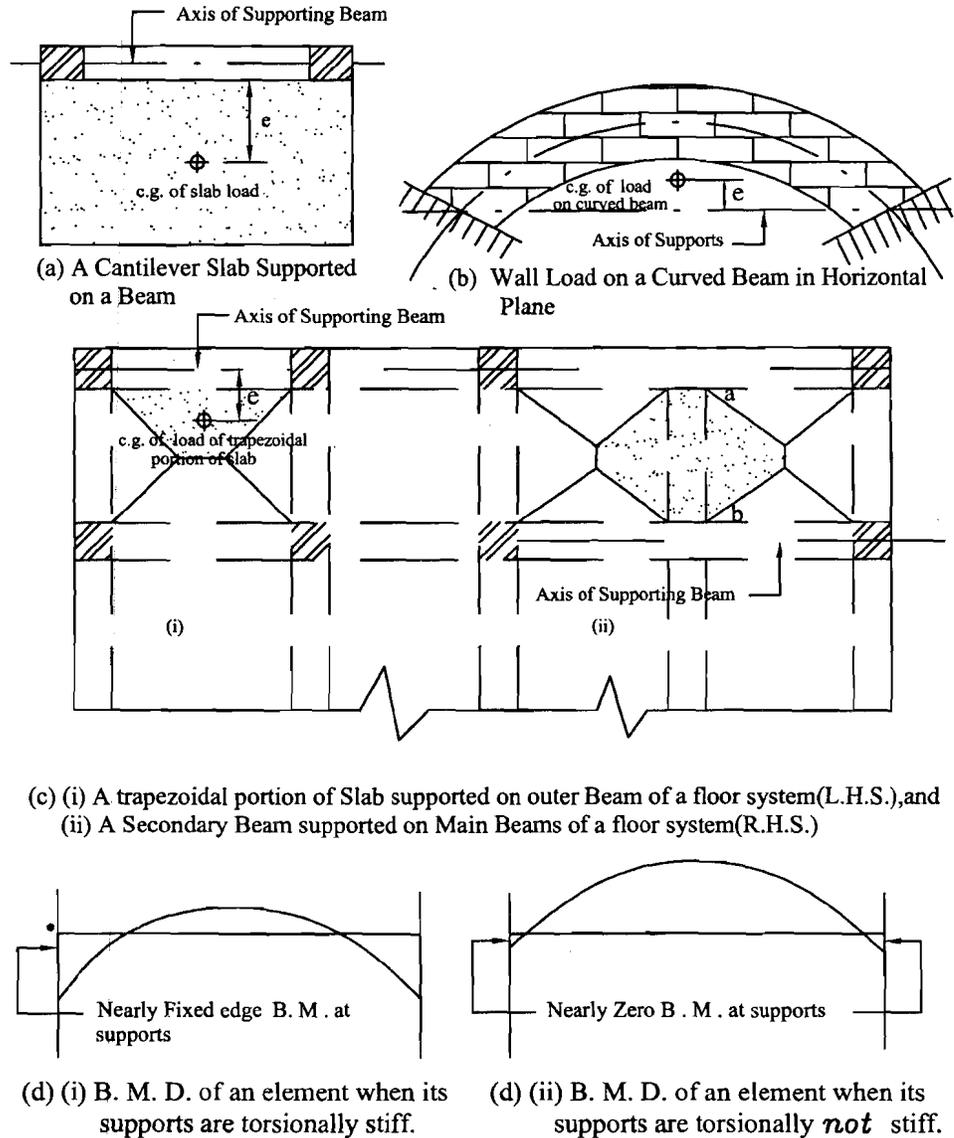
Figure 4.3 : Showing Torsional Moment due to Eccentric Loading on Supporting Element
