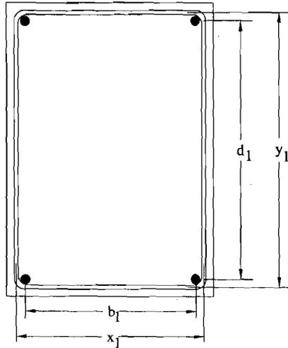
Figure 4.5 : Details of Transverse Reinforcement
