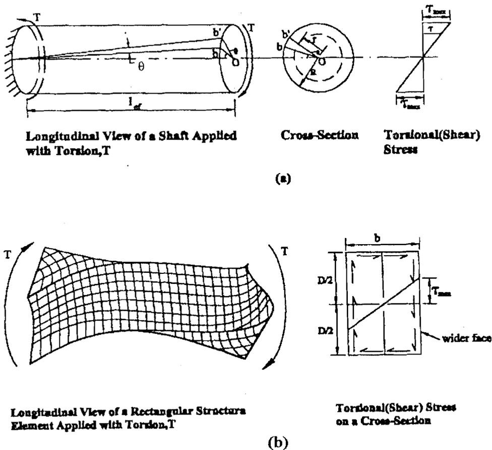
Figure 4.1 : A Shaft and a Rectangular Structural Element under Torsion, T
