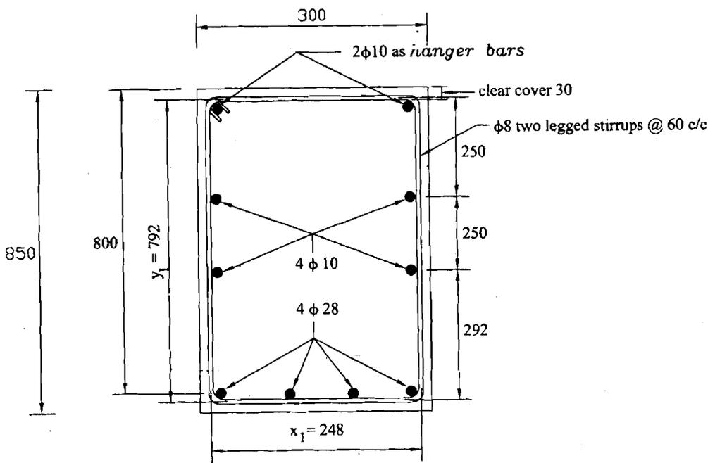
Figure 4.6 : Details of Reinforcement for Combined  $M_u$ ,  $V_u$ , and  $T_u$  having  $M_u < M_{u1}$
