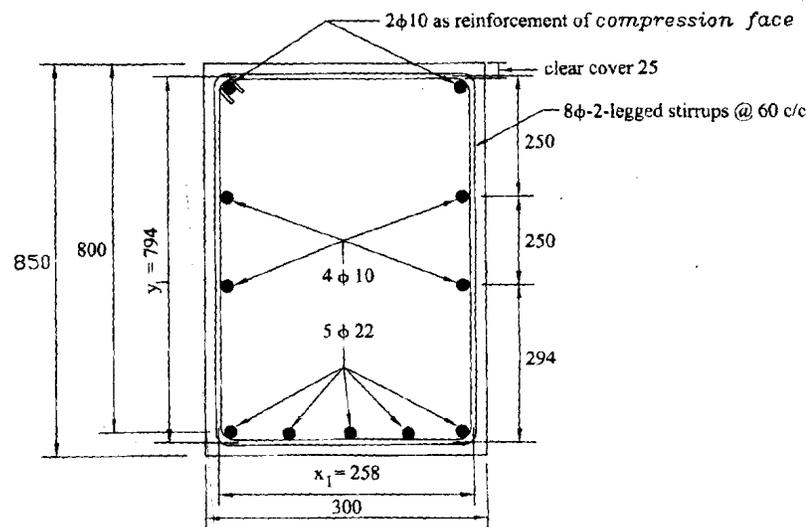
Figure 4.7 : Details of Reinforcements for Combined  $M_u$ ,  $V_u$ , and  $T_u$  having  $M_i > M_u$
