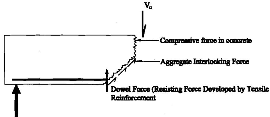
Figure 3.4 : Applied and Resisting Shear Forces
