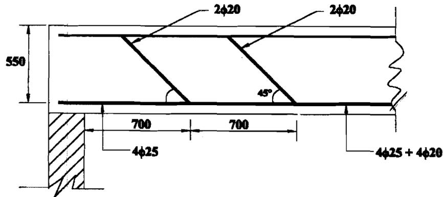
Figure 3.9 : Showing Bent-up Bars at Different Cross-Sections
