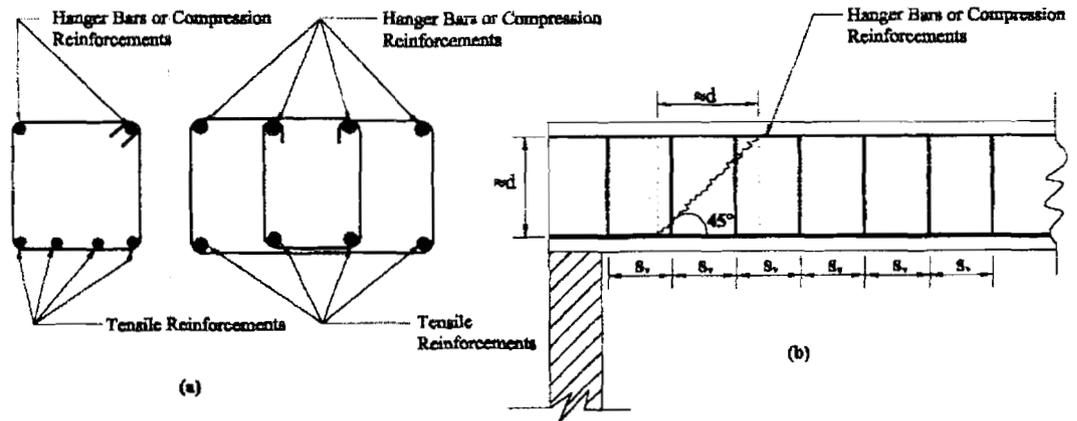
Figure 3.6 : Vertical Stirrups to Resist Shear Force
