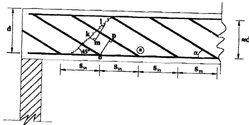
Figure 3.7 : Inclined Reinforcement to Resist a Part of Shear Forces
