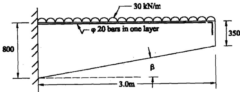
Figure 3.10 : Details of a Cantilever Beam
