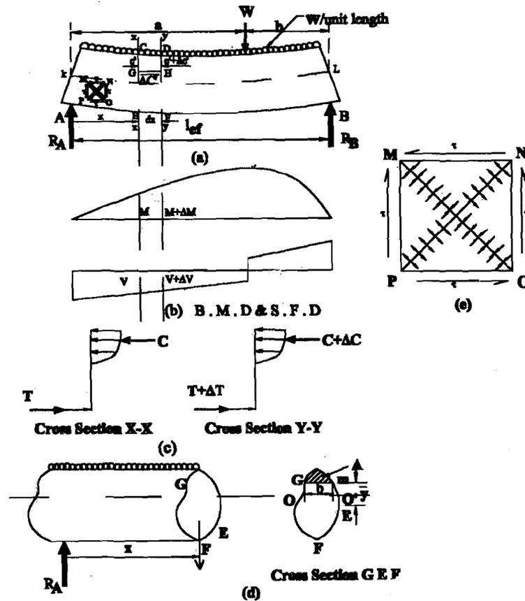
Figure 3.2 : Showing Effect of Varying B. M. D. Along a Beam
