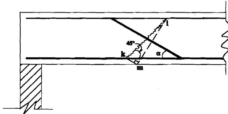
(a) Single or Group of Parallel Inclined Bars to Resist Shear at the Same Cross-Section
