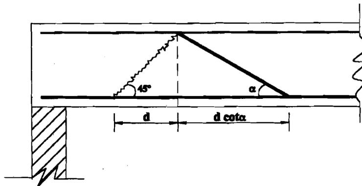
(b) Maximum Distance Between Bent-up Bars or Inclined Stirrups
