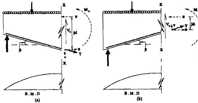
Figure 3.5 : Force Actions for Beams of Varying Depth
