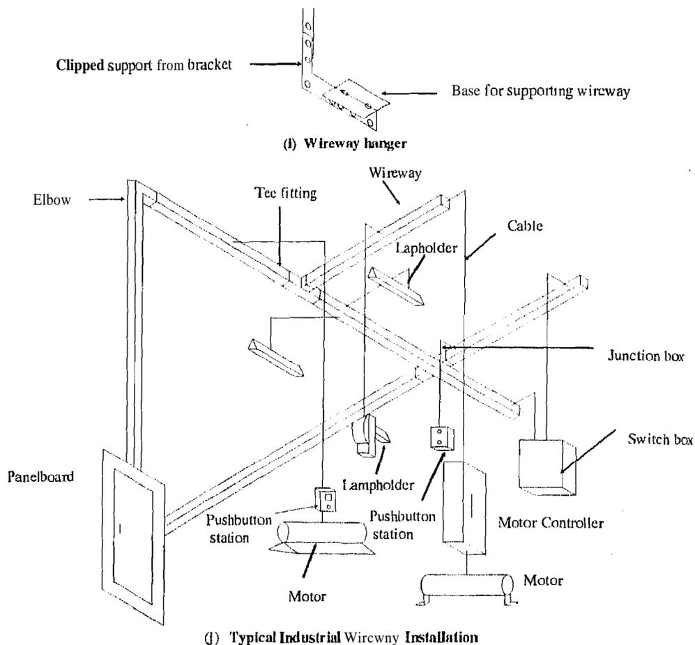
Fig 9.14 : Typical Industrial Wireway Installation
