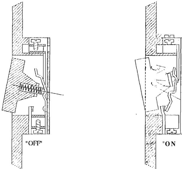
Rocker-operated switch mechanism, showing moving contact and spring-loaded ball and socket operation
