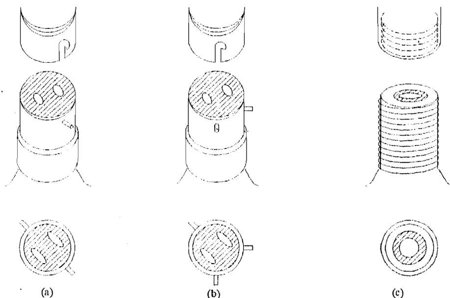
Fig. 9.8 Lamp Bolders bayonet Cap Type and Edison Screw Type.
