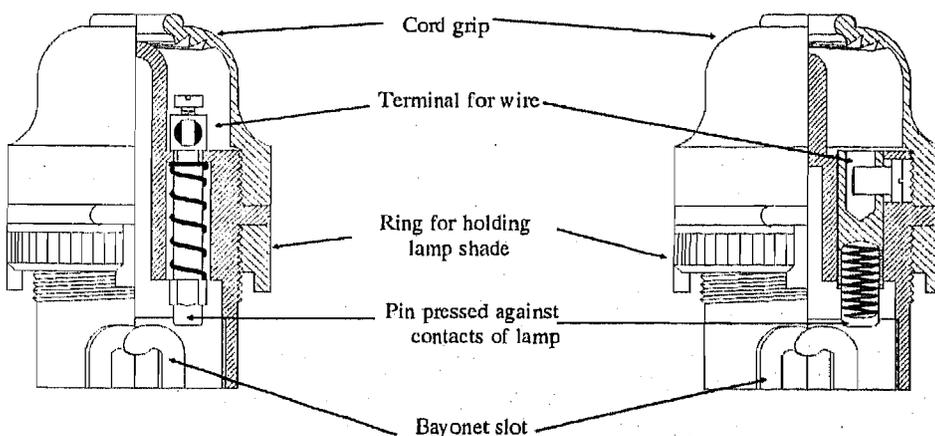
Fig. 9.6 Two Types of Pendant Lamp Holder, a Solid Plunger (left) and a Spring Plunger (right)
