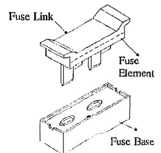
Fig. 9.12 Rewirable Fuse Unit
