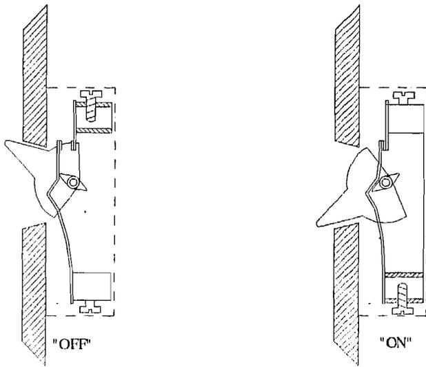
Tumbler operated lighting switch showing cam operated moving contact and operation of switch
