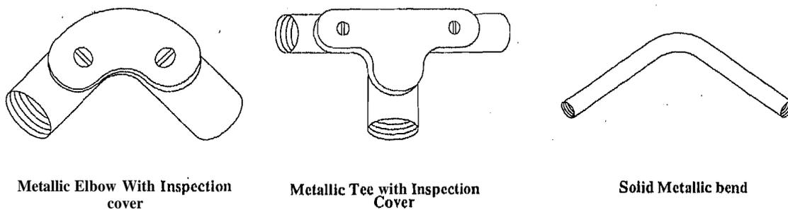
Fig. 9.4 Solid and Inspection types of Bends, Tee and Elbow.
