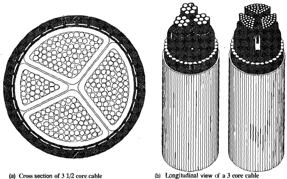
(a) Cross section of 3 1/2 core cable
