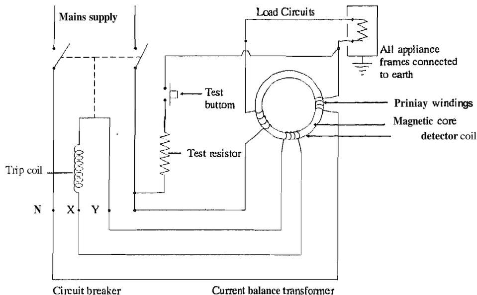
Fig. 9.16 : Current Operated Earth Leakage Circuit Breaker
