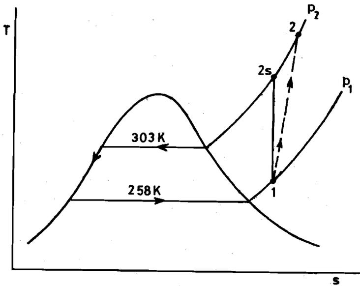
Figure 13.7 : Adiabatic compression on  $T$ - $S$  coordinates
