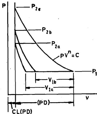
Figure 13.8 : Effect of pressure-on capacity
