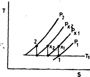
Figure 13.12 : Three stage compression with intercooling
