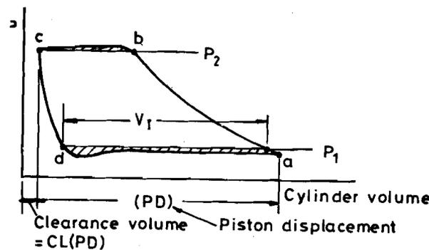
Figure 13.3 : Compressor Indicator Diagram
