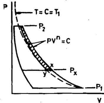
(b) Two-stage compression with intercooling
