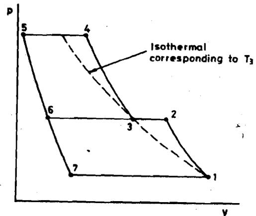
Figure 13.14 : Two-stage process
