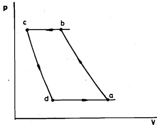
Figure 13.6 : Indicator diagram
