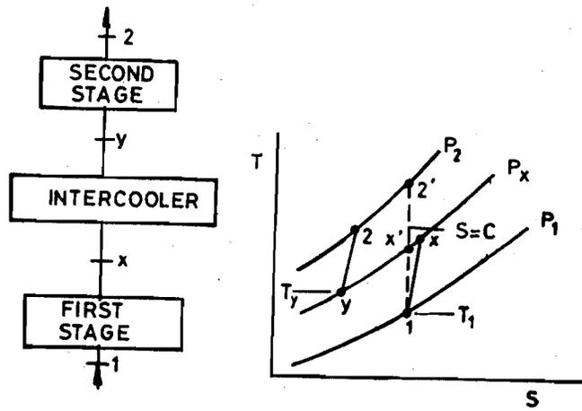
Figure 13.11 :  $T-s$  plot of two-stage compression process
