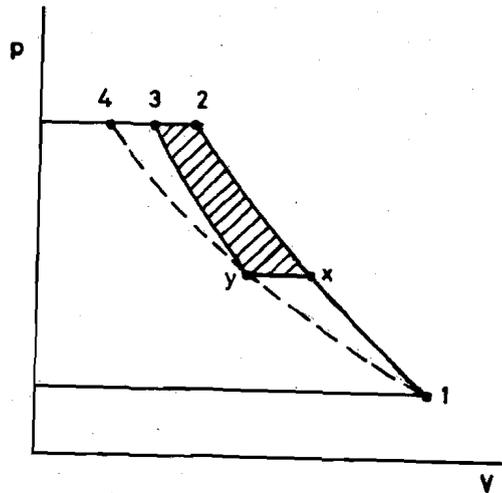
Figure 13.13 : Indicator diagram of two-stage compressor
