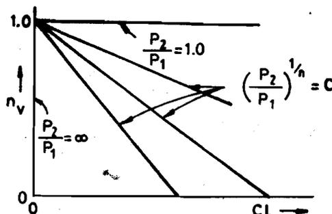
Figure 13.5 : Effect of clearance on volumetric efficiency
