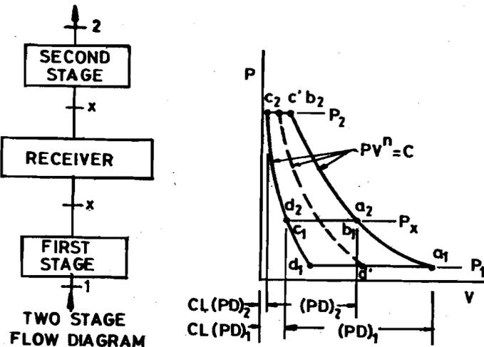
Figure 13.9 : Two-stage compression
