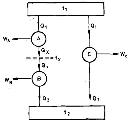
Fig. 7.5: Reversible heat engines, *A*, *B* and *C* operating between  $t_1$  and  $t_2$
