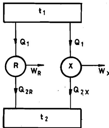
Fig. 7.2: Heat engines  $R$  and  $X$  operating between  $t_1$  and  $t_2$
