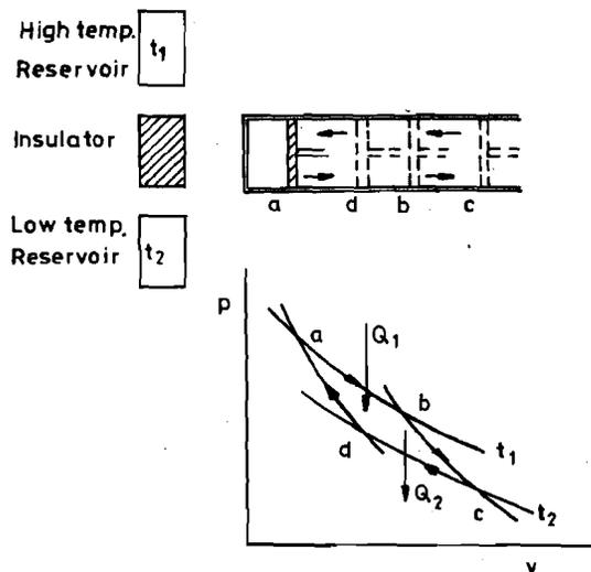
Fig. 7.4: Carnot Heat Engine
