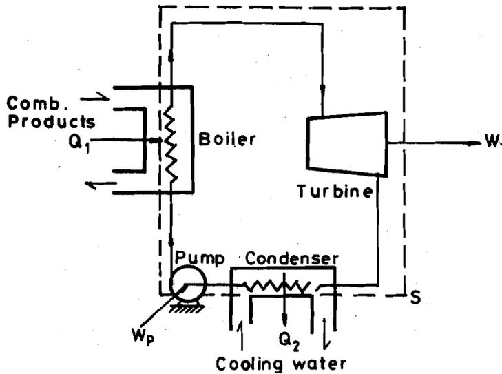
Fig.6.1 : Schematic of steam power plant
