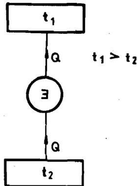
Fig.6.7 : Impossible reversed heat engine (heat pump with infinite COP)
