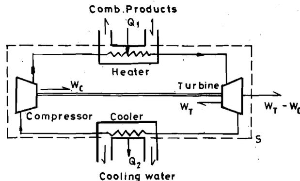
Fig.6.2 : Schematic of closed cycle gas turbine power plant
