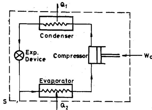
Fig.6.3 : Schematic of a refrigerator/heat pump
