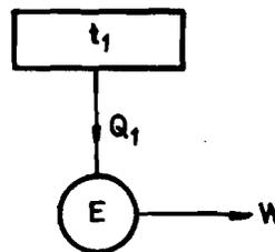
**Fig. 6.6 : Impossible direct heat engine (PMM II or 100% efficient engine)**
