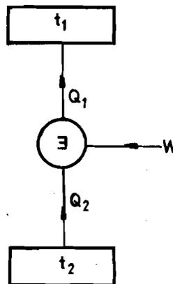
Fig.6.5 : Symbolic representation of a reversed heat engine
