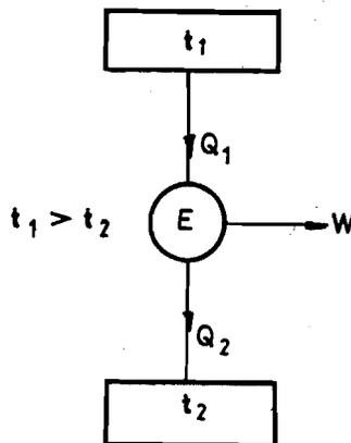
Fig.6.4 :Symbolic representation of direct heat engine
