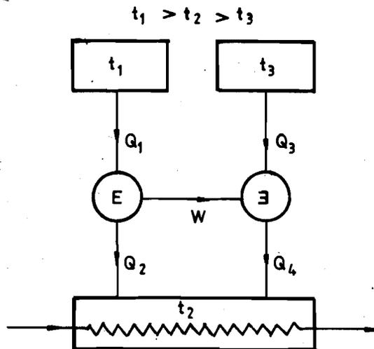
Fig.6.10 : Heat pump driven by the heat engine
