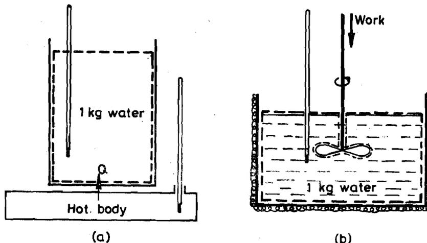
Figure 4.1 : Experiments in which the same effect is achieved (a) by Heat and (b) by Work
