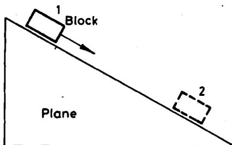
Figure 4.5 : Block sliding down a rough inclined plane
