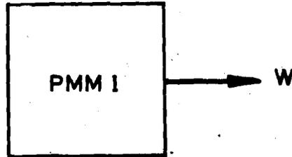
Figure 4.6 : Perpetual-Motion Machine of The First Kind
