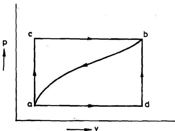
Figure 4.2 : Path of two cyclic processes passing through two common state points
