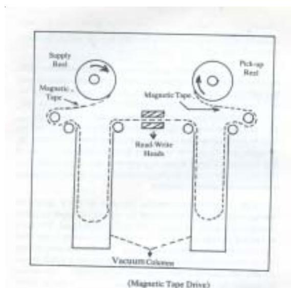
of small particles of iron oxide mixed with a binding material. Data is stored as a magnetic pattern of bits on **tracks** that run the length of the tape. A magnetic spot represents a 1; no magnetic spot represents a 0.
