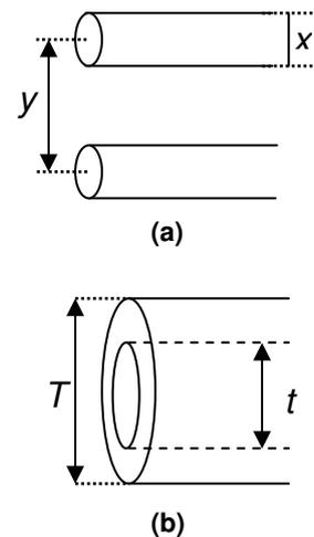
**Fig. 4.6: a) Parallel wires; and b) coaxial cable**
