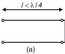
This is equivalent to an impedance of an inductor.
