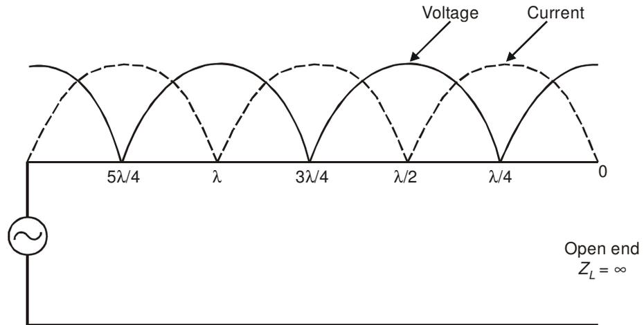
Fig. 4.11: Standing wave patterns of current and voltage on the open ended transmission line
