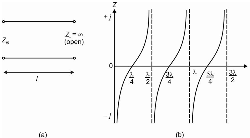
You must remember here that practically, under  $Z_{open}$  case the impedance is not infinite. The free space acts as a load here with impedance of  $377 \Omega$ . Hence in reality,  $Z_L = \infty$  is actually  $Z_L \gg Z_0$ .
