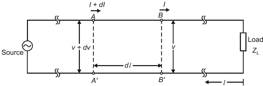
Fig.4.5: Current and voltage relations in a short segment of transmission line
