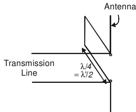
Fig. 4.21:  $\lambda/4$  Shorted line as low pass filter
