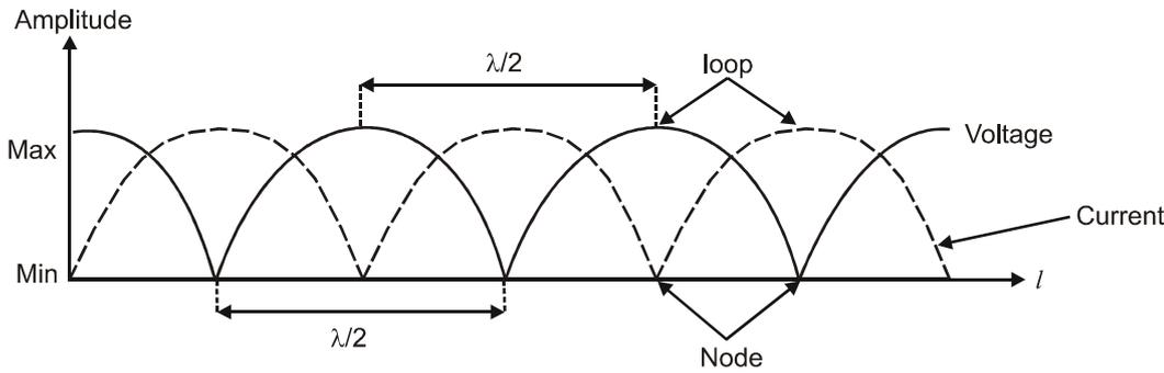
Fig.4.8: Standing wave pattern in a loss-less line
