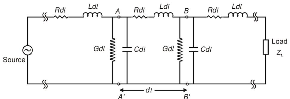
Fig.4.4: Lumped component representation of transmission line
