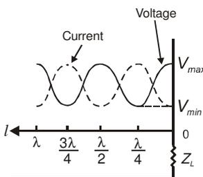
Fig. 4.15: Standing wave pattern for  $Z_L = R_L > Z_0$
