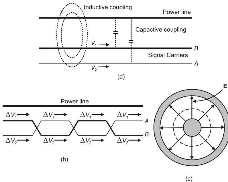
Fig. 4.2: a) Noise coupling in parallel conductor transmission line; b) noise reduction in twisted pair transmission line; and c) electric field confinement in coaxial cable
