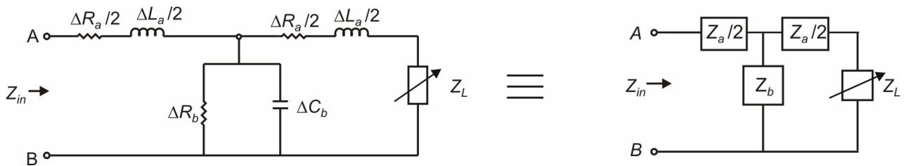
**Fig. 4.9: Lumped equivalent circuit of finite line section**
