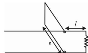
Fig. 4.19: Single stub impedance matching
