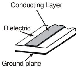
Fig. 4.3: Construction of Microstripline
