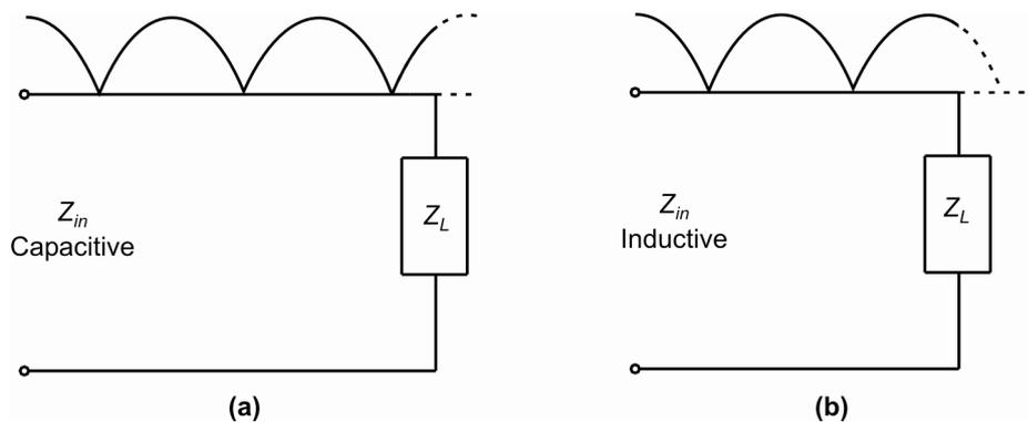
Fig. 4.16: Voltage distributions beyond the load point
