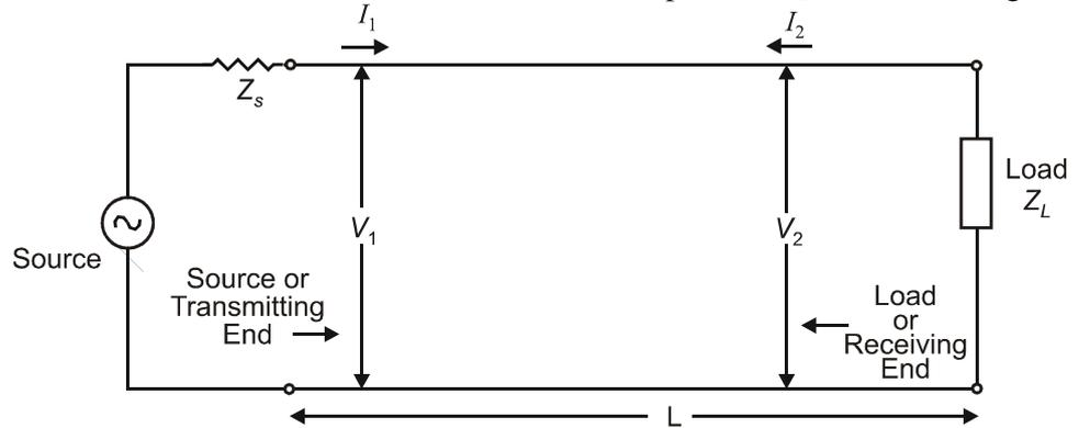
Fig. 4.7: Transmission line terminated in a load impedance
