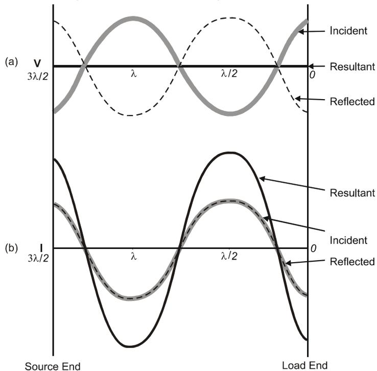
Fig. 4.24: a) voltage and b) current wave on short-circuited transmission line
