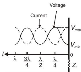
Fig. 4.14: Standing wave pattern for  $Z_L = R_L < Z_0$
