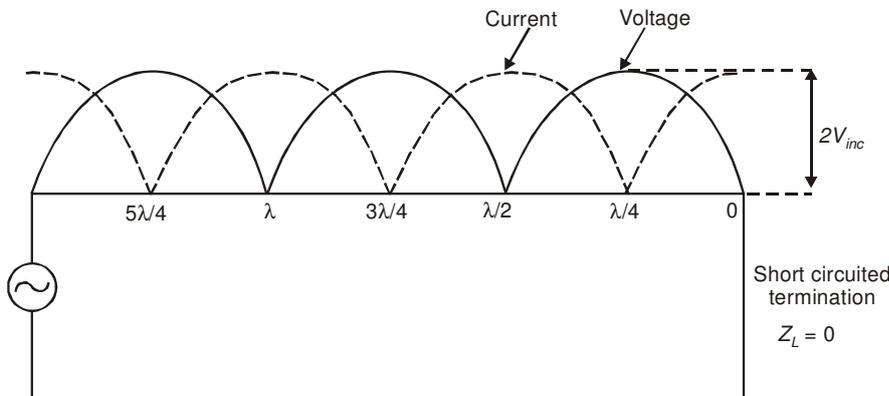
**Fig. 4.13: Standing wave patterns in a short circuited transmission line**
