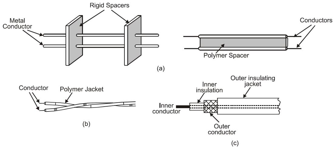
Fig. 4.1: Transmission Lines a) Parallel conductors; b) twisted pair and c) coaxial cable
