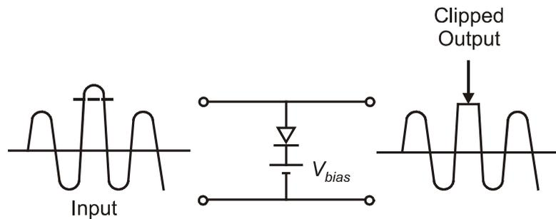
Fig. 2.15: Biased diode clipper circuit
