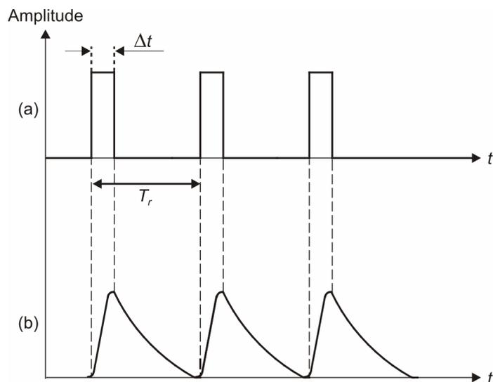
Fig. 2.9: Repetitive pulse signal: a) input to system and b) output of system
