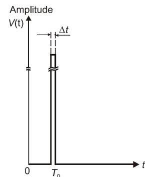
Fig. 2.7: Transient pulse waveform
