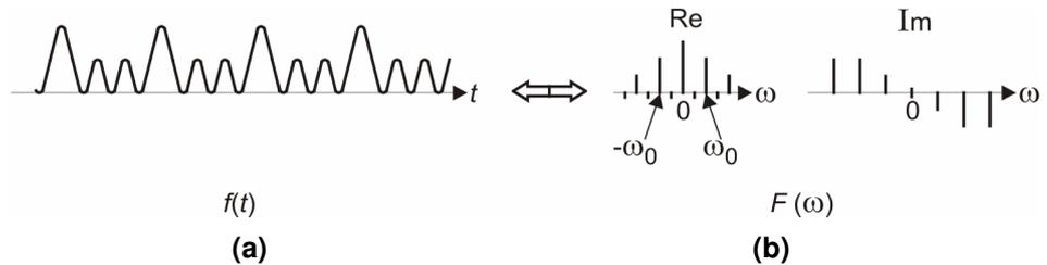
Fig. 2.17: a) Time; and b) frequency domain signal
