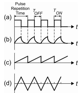
Fig. 2.11: a) Square wave input; b) System response; c) Saw tooth; and d) Triangular waveform
