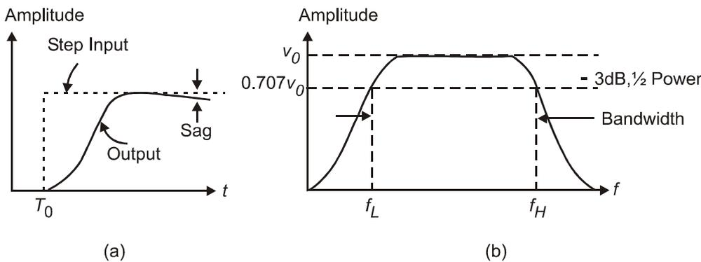
Fig. 2.12: a) Time domain response of system using step input; and b) frequency response of system using sine wave input
