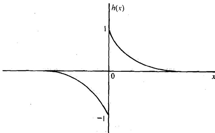
Fig.10.7: The function  $e^{-px}$  for  $x > 0$  and its odd continuation for  $x < 0$ , for some (positive) value of  $p$ .
