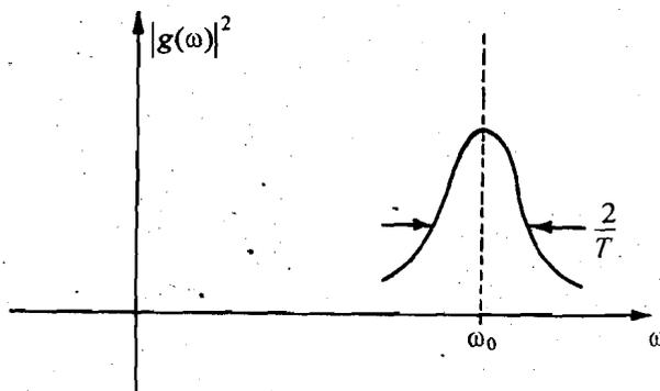
Fig.10.5: Spectrum of radiated energy
