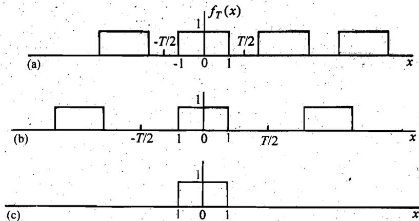
**Fig.10.1:** (a) A rectangular periodic pulse with width 2 and period  $T$ ; (b) the same pulse with a larger  $T$ ; (c) as  $T$  is made infinitely large, there is only one pulse, giving an aperiodic function.
