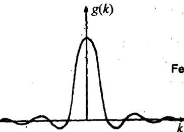
Fig.10.3: Fourier transform of a single square pulse.
