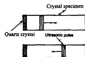
**Fig.6.9:** A pulse of sound is generated by piezoelectric transducer; the pulse undergoes successive reflections and is detected each time it reaches back to the transducer.
