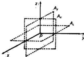
Fig.6.2: Three elements of area at a reference point P
