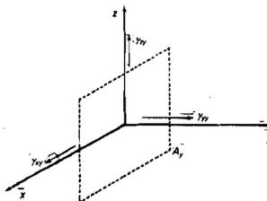
Fig.6.3: Stress components  $\gamma_{xy}$ ,  $\gamma_{yy}$  and  $\gamma_{zy}$  on an element of area  $A_y$
