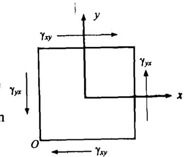
Fig.6.4: For a body in static equilibrium,  $\gamma_{yx} = \gamma_{xy}$ . The sum of forces in the  $x$ -direction as well as in  $y$ -direction is zero. The total torque about the origin (say  $O$ ) is zero if  $\gamma_{yx} = \gamma_{xy}$ .
