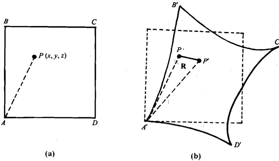
Fig.6.6: a)  $ABCD$  is cross-sectional view of a three dimensional body before deformation; and b)  $A'B'C'D'$  is deformed section
