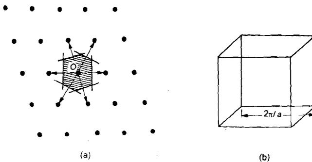
Fig.3.16: a) FBZ of 2-D oblique reciprocal lattice; and b) FBZ of 3-D sc reciprocal lattice
