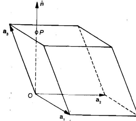
Fig.3.8: Volume of a unit cell
