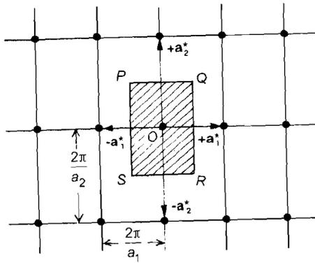
Fig.3.12: The FBZ of a rectangular reciprocal lattice
