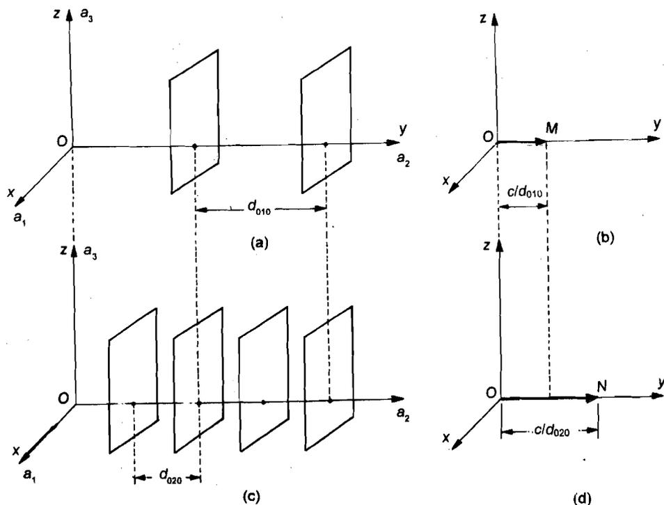
Fig.3.2: a) Family of  $(010)$  planes in direct lattice; b) reciprocal lattice point corresponding to  $(010)$  planes; c) family of  $(020)$  planes in direct lattice; and d) reciprocal lattice point corresponding to  $(020)$  planes
