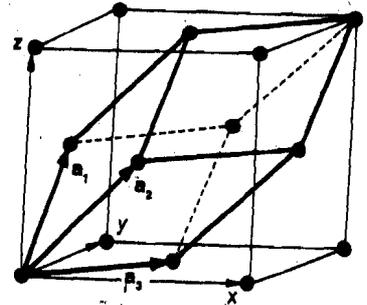
Fig.3.11: Primitive cell in fcc lattice
