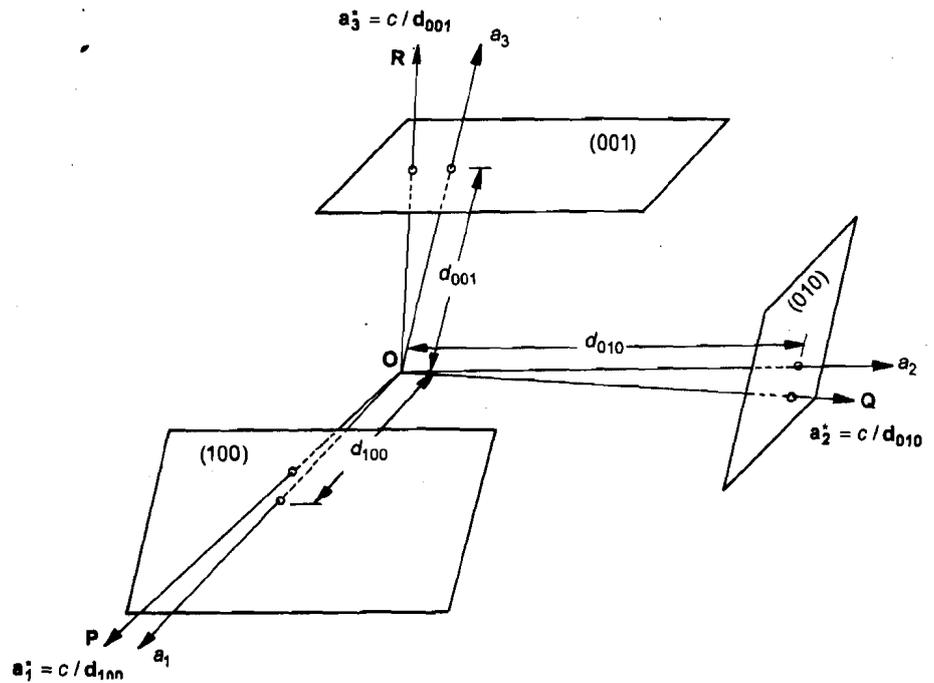
Fig 3.5: Construction of 3-D reciprocal lattice
