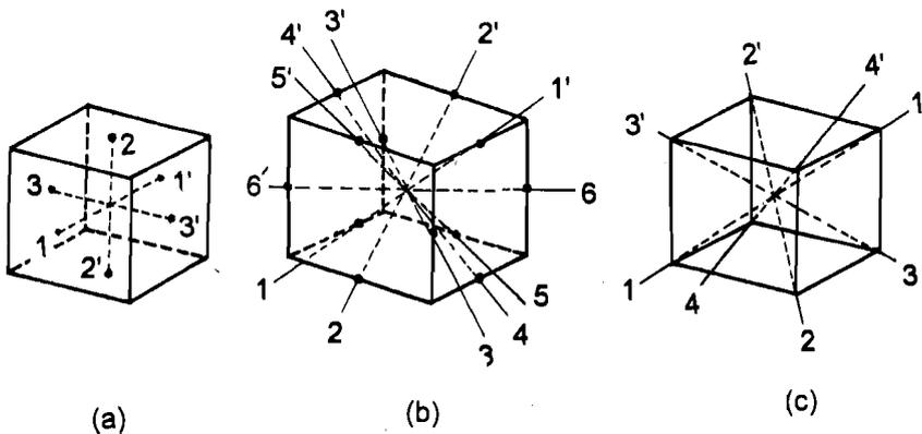
Fig.1.16: Rotation axes of a cube
