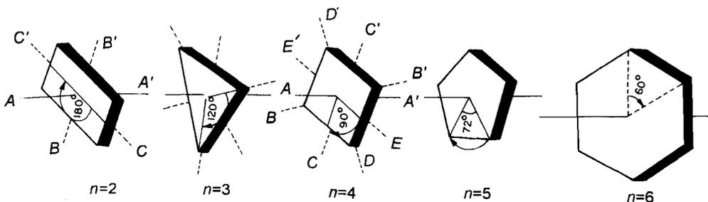
Fig.1.15: Objects with different folds of rotation axes symmetry
