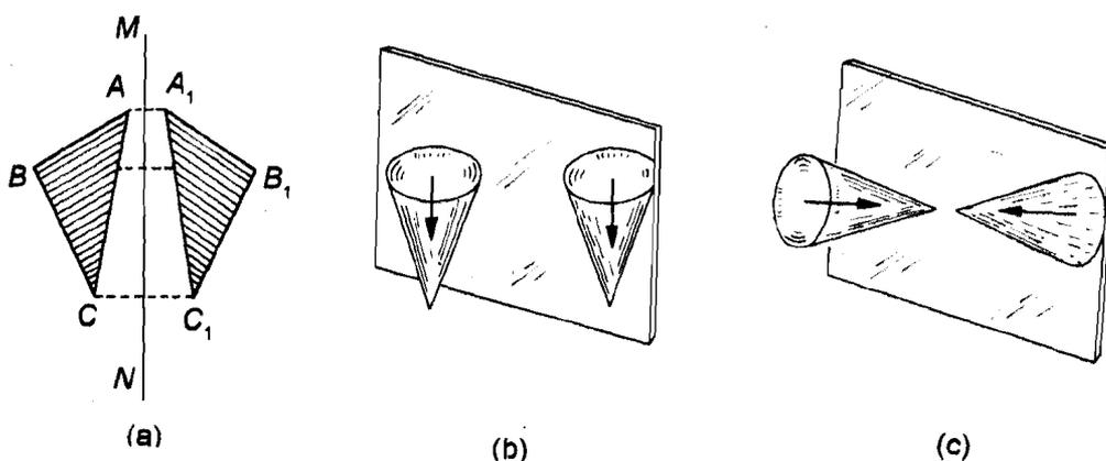
Fig.1.1: Reflection symmetry for a) a 2-D object; b) a 3-D object placed vertically; and c) placed horizontally
