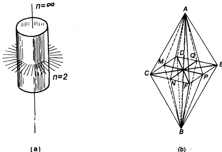
Fig.1.17: Rotation axes of a) a cylinder; and b) a body made of two regular pyramids
