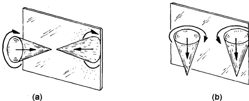
Fig.1.6: Reflection of a) a horizontal cone; and b) a vertical cone
