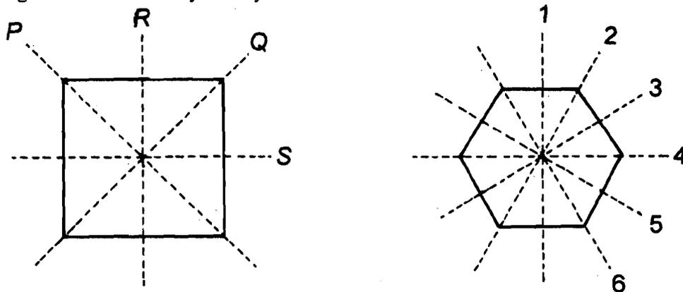
Fig.1.4: Axes of symmetry for a square and a hexagon
